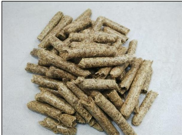
**Figure 2a** Oil palm Empty Fruit Bunch (OPEFB) briquettes.
