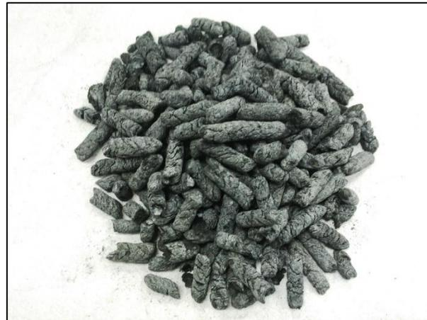
**Figure 2b** Biochar of OPEFB briquettes after gasification
