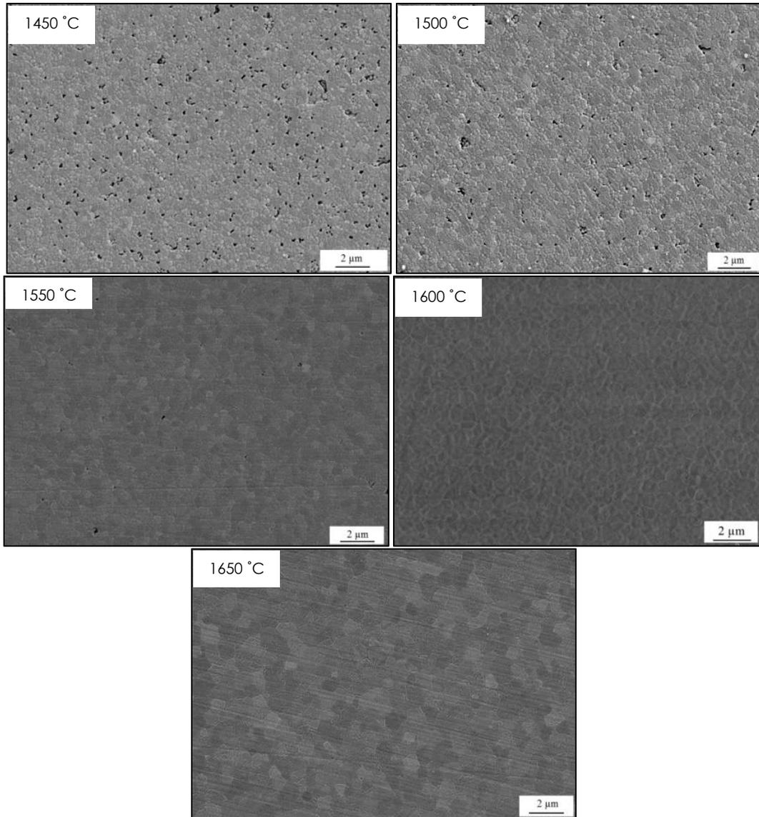
Figure 4 SEM images of YSZ specimens sintered at different temperatures
