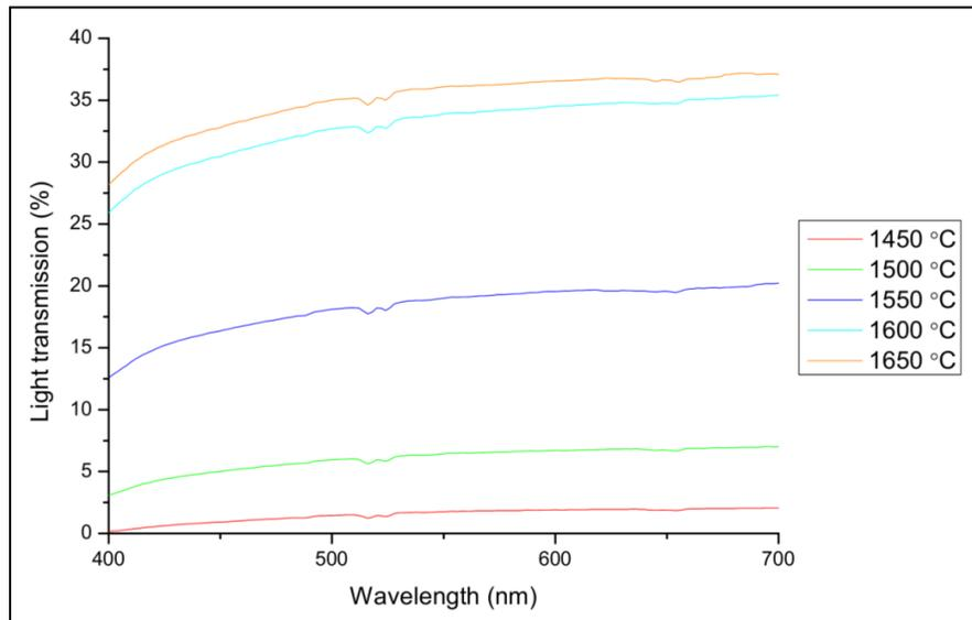
Figure 5 Light transmissions of YSZ specimens sintered at different sintering temperatures
