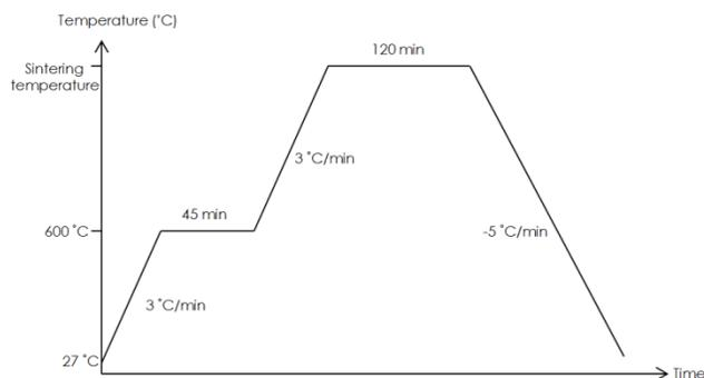
Figure 2 Sintering profile
