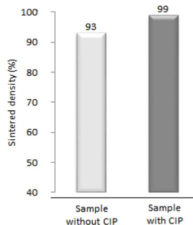
Figure 3 Density of Y-TZP samples with and without CIP
