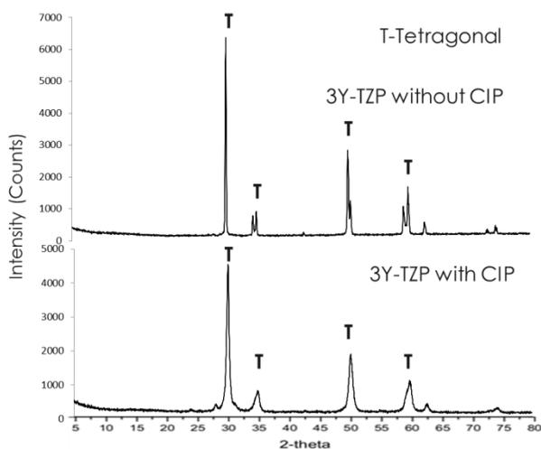
Figure 7 XRD results of Y-TZP samples with and without CIP
