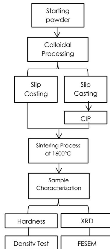
Figure 1 Flow diagram of sample preparation
