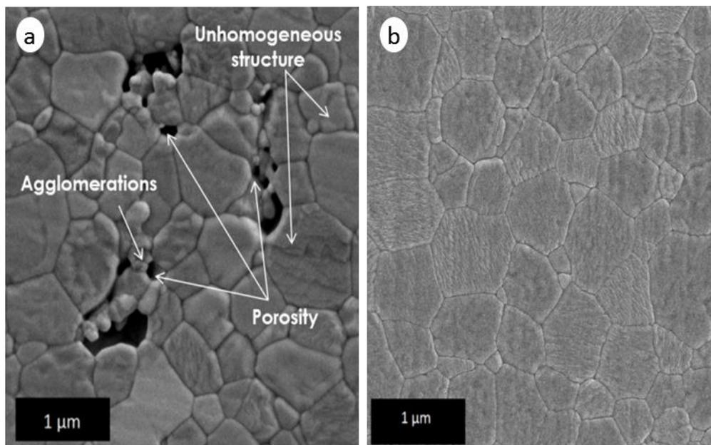
**Figure 5** FESEM micrograph of 3Y-TZP without CIP (a) and with CIP (b)
