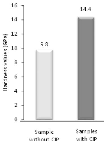
**Figure 4** Hardness of Y-TZP samples with and without CIP
