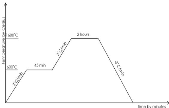
Figure 2 The sintering process scheme
