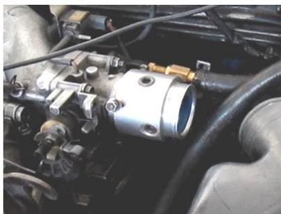
**Figure 5** The mixer used in this study, with 30, 35, and 40 mm of venturi diameter
