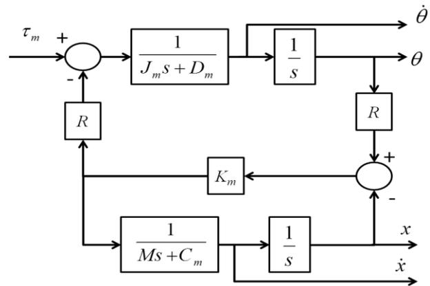
Figure 3 Block diagram of ball screw mechanism
