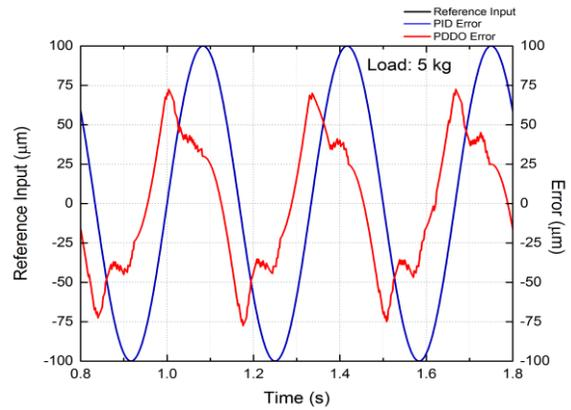
**Figure 13** Experimental tracking results of PDDO and PID controller when subjected to 5 kg load in 3 Hz with 100  $\mu\text{m}$  sinusoidal input
