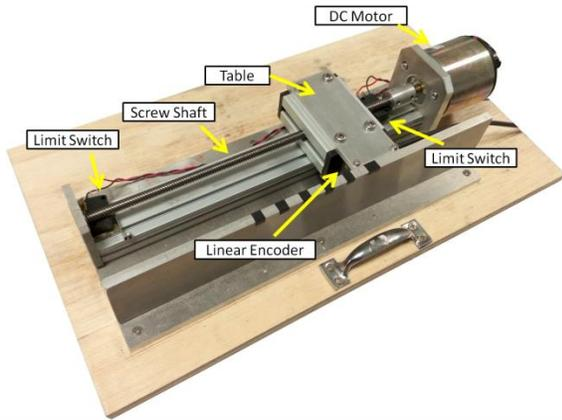
Figure 1 Ball screw mechanism driven by DC motor
