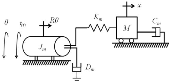
Figure 2 Free body diagram of ball screw mechanism
