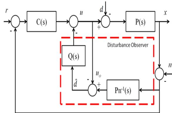
Figure 6 Block diagram of PDDO controller
