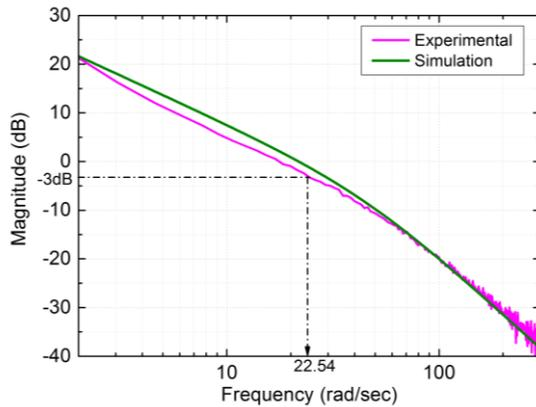
Figure 5 Comparisons of open loop frequency response for experimental and simulation results
