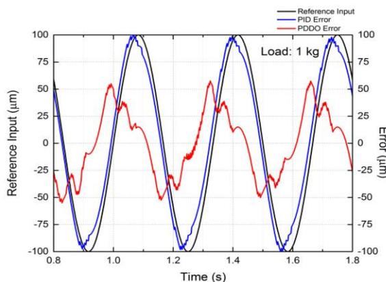
**Figure 12** Experimental tracking results of PDDO and PID controller when subjected to 1 kg load in 3 Hz with 100  $\mu\text{m}$  sinusoidal input
