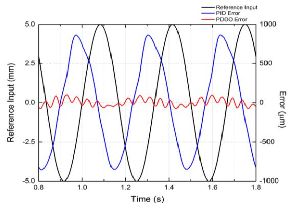
Figure 9 Experimental tracking results of the PDDO controller and PID controller at sinusoidal input of 3 Hz and 5 mm amplitude
