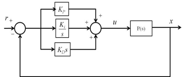
Figure 8 Control structure of PID controller
