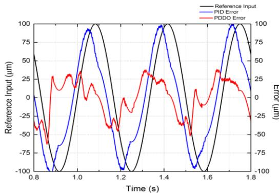
**Figure 11** Experimental tracking results of the PDDO controller and PID controller at sinusoidal input of 3 Hz and 100  $\mu\text{m}$  amplitude
