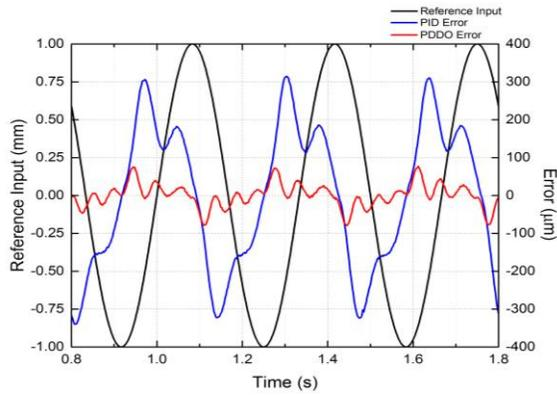
**Figure 10** Experimental tracking results of the PDDO controller and PID controller at sinusoidal input of 3 Hz and 1 mm amplitude
