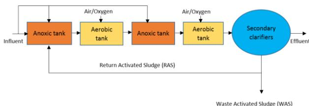
**Figure 3** Bonus RSTP's activated sludge process
