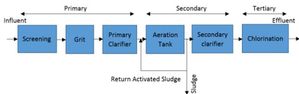
**Figure 1** Block diagram of wastewater treatment process
