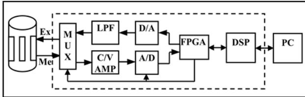
Figure 2 Digital ECT system architecture [17]
