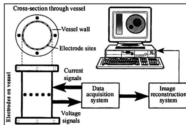
Figure 1 Schematic diagram of an ERT system
