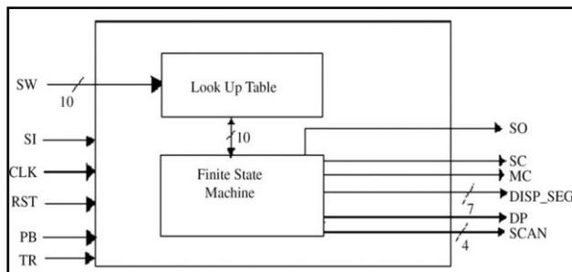
Figure 7 VHDL model of the proposed system [35]
