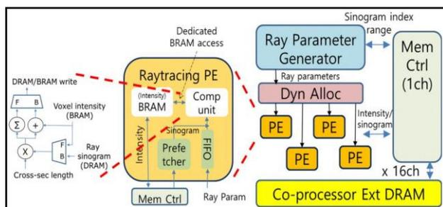
Figure 5 The architecture of the proposed system [27]
