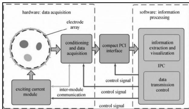
Figure 4 Structure of the ERT system [23]
