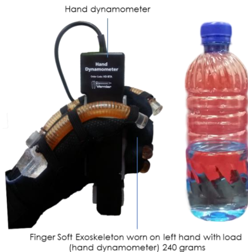
Figure 7 Standard position of hand grip test measurement. The hand dynamometer was weighted as 240 grams equivalent to 240 ml bottled mineral water.
