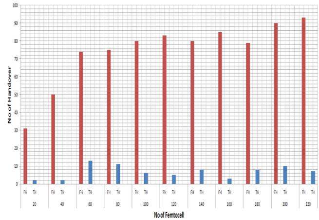
Figure 7 Number of handovers versus number of deployed femtocells
