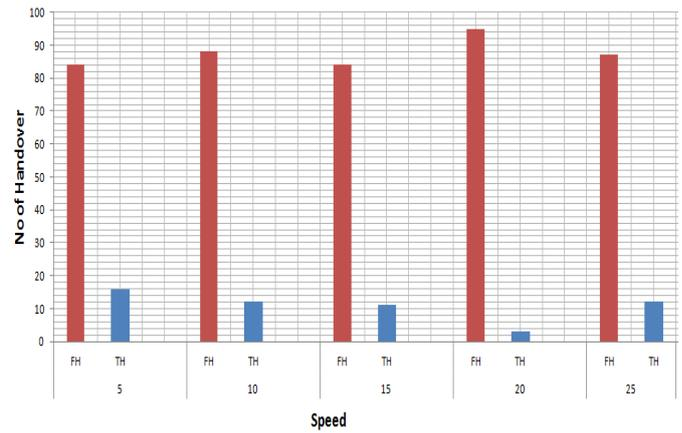
Figure 3 Number of handovers versus Speeds of UE for random movement. FH= femtocell handover TH=Traditional handover
