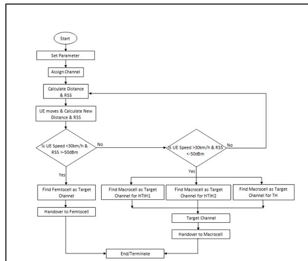
Figure 1 The workflow of proposed handover scheme
