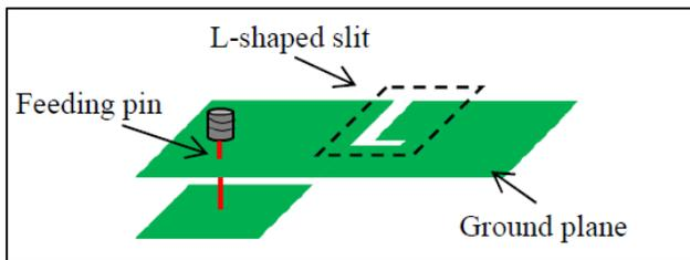
Figure 4 Structure for dual-mode antenna [6]
