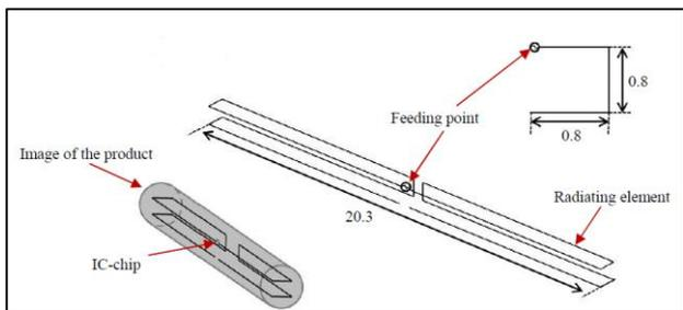
Figure 7 Configuration of the antenna [10]
