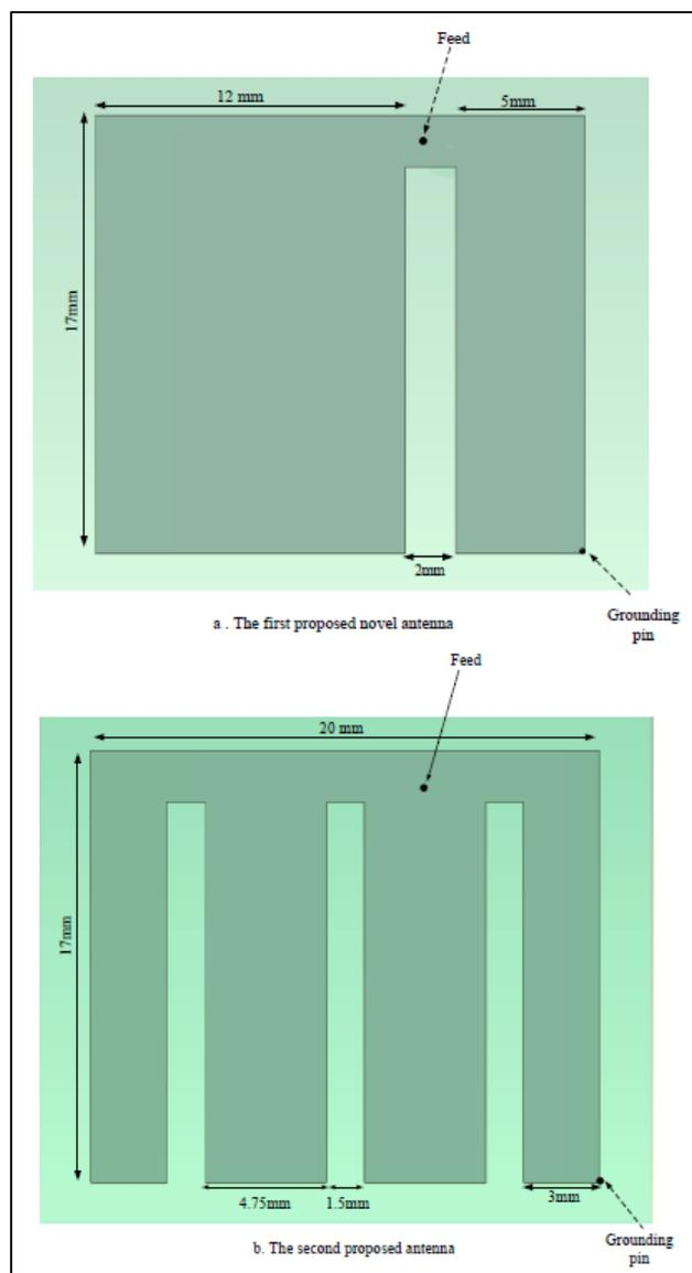
**Figure 12** Two proposed antenna design for SAR reduction [14]
