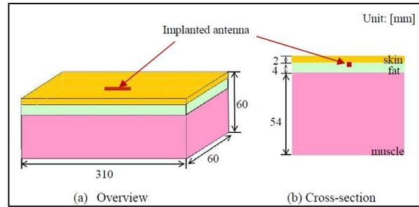
Figure 8 Numerical model of implanted antenna [10]
