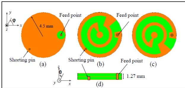
Figure 6 Proposed antenna geometry [3]
