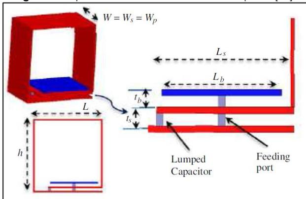
Figure 11 Front and magnified view of ECLA structure [13]
