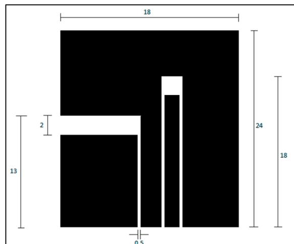
Figure 9 CPW fed antenna structure [11]
