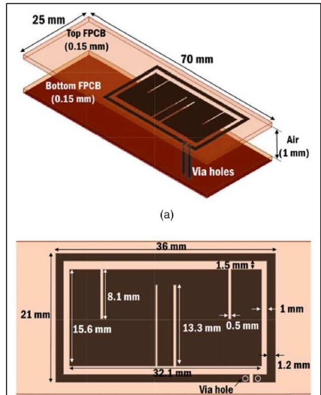
Figure 5 Geometry and dimension of the patch antenna [8]
