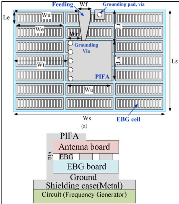
Figure 3 PIFA geometry (top and side view) [5]
