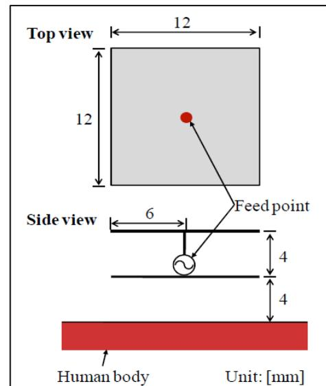
**Figure 2** Antenna geometry [4]
