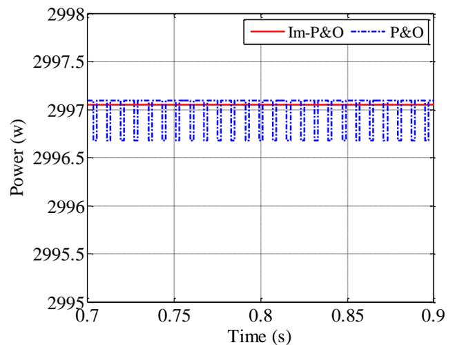
Figure 6 Steady state responses of the Im-P&O and conventional P&O
