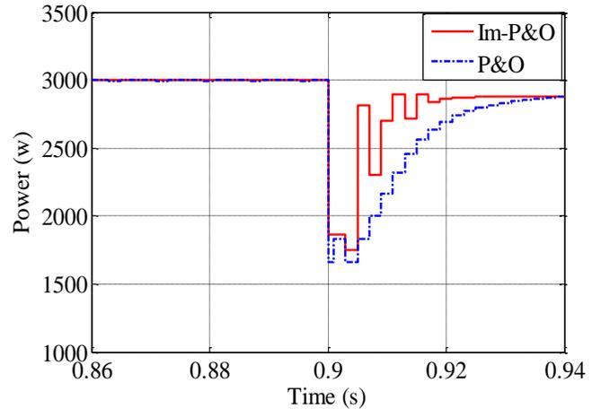
Figure 14 Response of Im-P&O and P&O for the step temperature change
