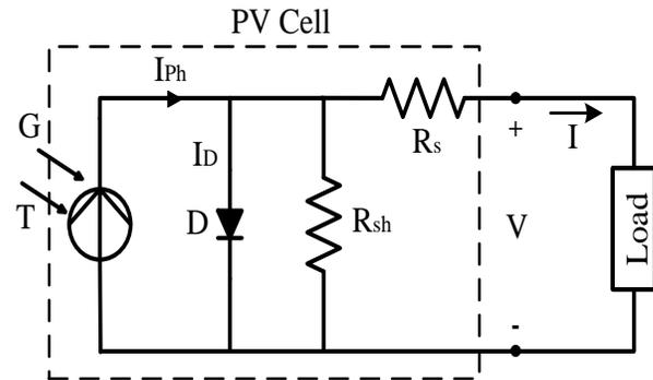
Figure 1 Electrical equivalent circuit of PV cell
