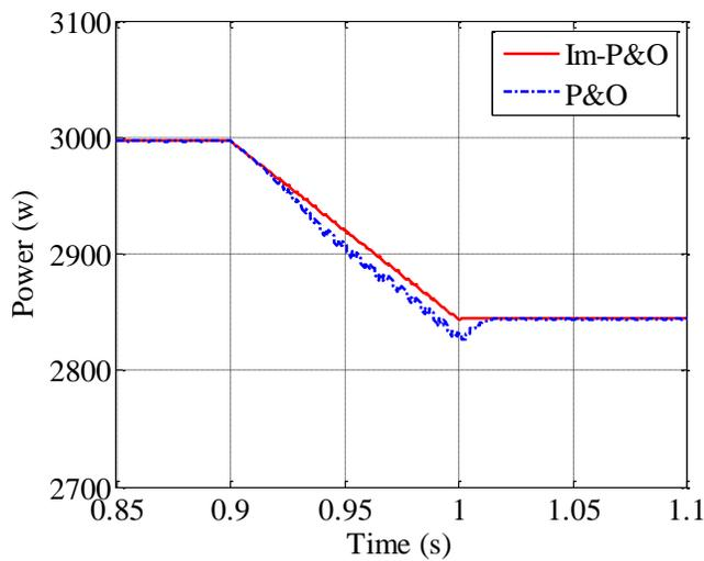
Figure 8 Response of Im-P&O and P&O for the ramp irradiance change
