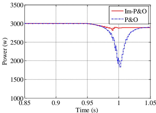
Figure 12 Response of Im-P&O and P&O for the ramp temperature change
