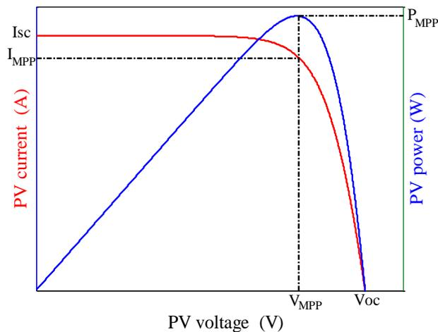
Figure 2 P-V curve of a PV module
