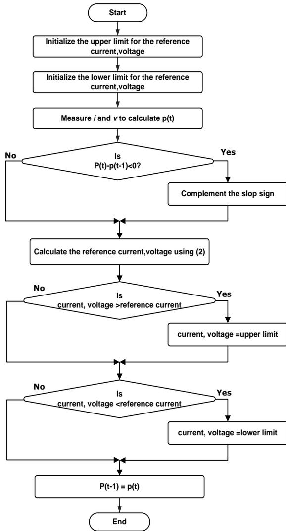
Figure 4 Flowchart of the proposed Im-P&O algorithm
