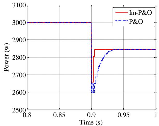
Figure 10 Response of Im-P&O and P&O for the step irradiance change
