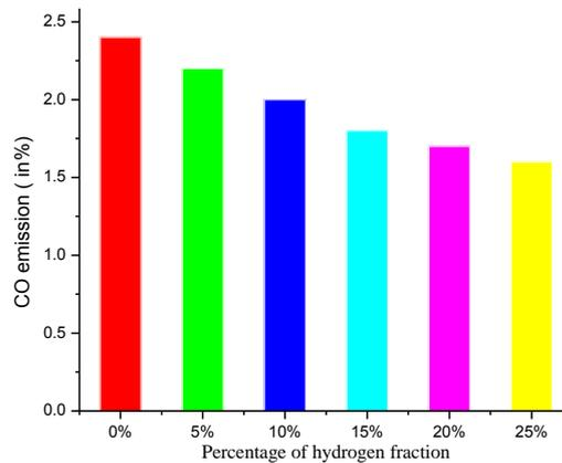
**Fig. 7. Variation of CO emission with various hydrogen fractions.**
