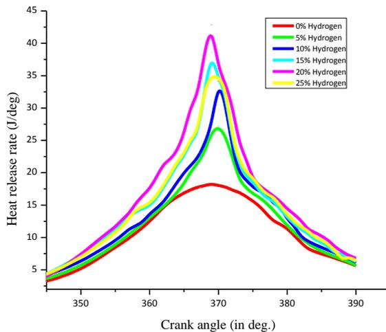
**Fig. 4. Variation of net heat release with various hydrogen fractions.**
