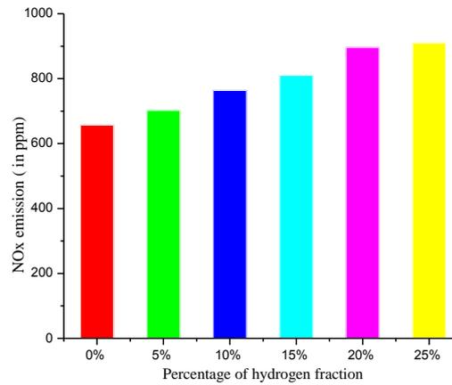
**Fig. 6. Variation of  $\text{NO}_x$  emission with various hydrogen fractions.**
