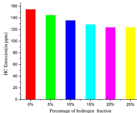
**Fig. 5. Variation of HC emission with various hydrogen fractions.**
