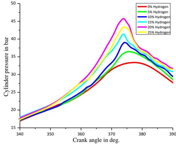
**Fig. 3. Variation of cylinder pressure with various hydrogen fractions.**
