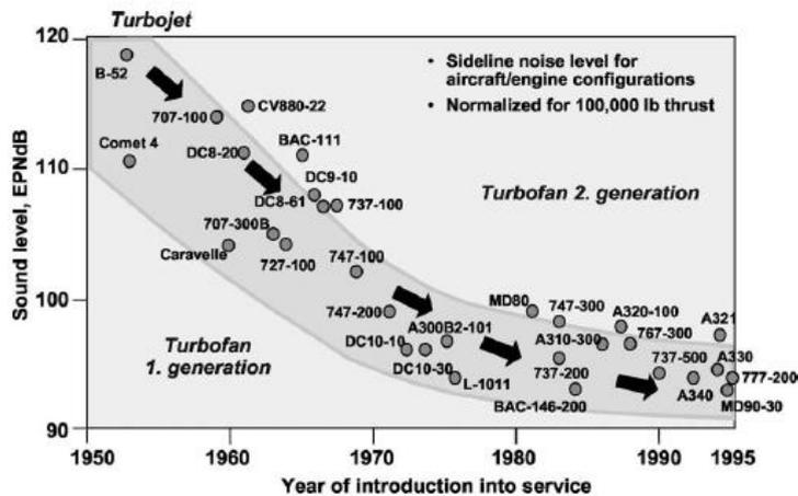
**Fig. 1. Reduction of aircraft noise with respect the year of entry into service [12].**
