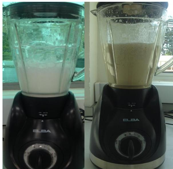
**Figure 1** Shakers used for foam stability (a) without oil (b) with oil
