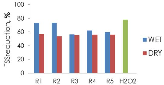
Figure 10 Percentage of TSS reductions for wet and dry sludge as compared with blank
