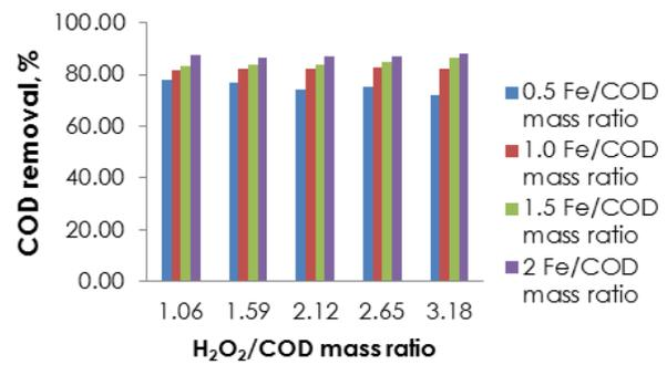
Figure 3 Percentage of COD removals in different H<sub>2</sub>O<sub>2</sub> /COD mass ratio and different Fe/COD mass ratio
