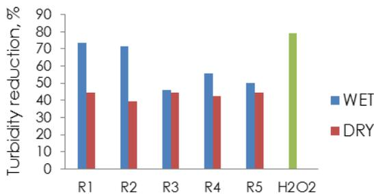
Figure 9 Percentage of turbidity reduction for wet and dry sludge as compared with blank
