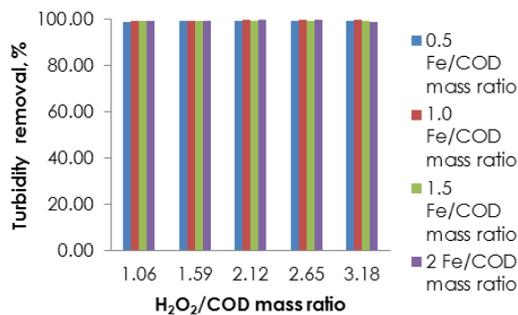
**Figure 5** Percentage of turbidity reduction in different  $\text{H}_2\text{O}_2/\text{COD}$  mass ratio and different Fe/COD mass ratio
