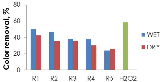
Figure 8 Percentage of Color removals for wet and dry sludge as compared with blank
