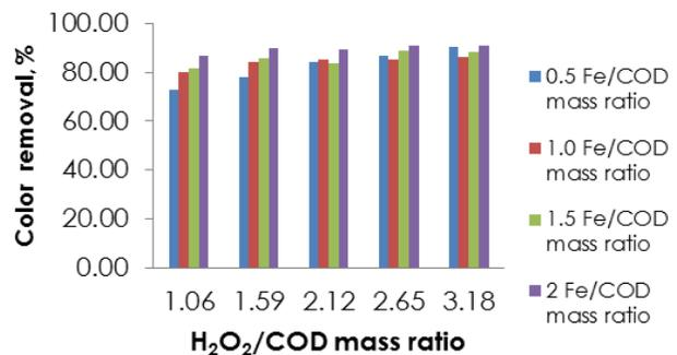
Figure 4 Percentage of Color removals in different H<sub>2</sub>O<sub>2</sub>/COD mass ratio and different Fe/COD mass ratio
