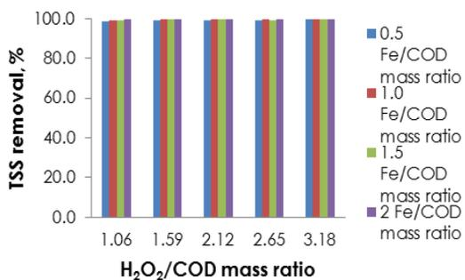
**Figure 6** Percentage of TSS reductions in different  $\text{H}_2\text{O}_2/\text{COD}$  mass ratio and different Fe/COD mass ratio
