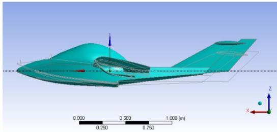
Figure 10 Model geometry with  $\alpha = 0^\circ$  without towing Tank
