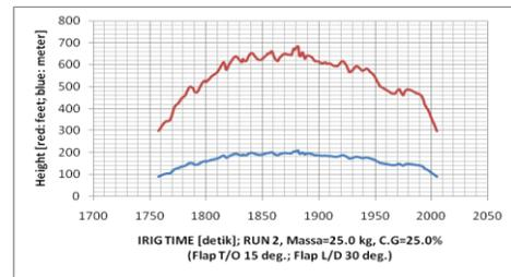
Figure 19 The Height, h of Unmanned Aerial Vehicle “Alap alap” flight testing data during takeoff
