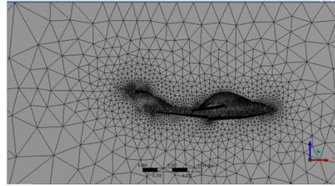
Figure 12 Meshing of the model with  $\alpha = 0^\circ$
