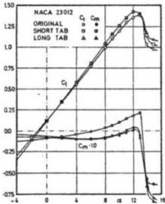
Figure 2 The aerodynamics characteristic of NACA 23012 airfoil (original and modification)<sup>[17]</sup>
