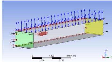
Figure 13 Boundary condition of the remote control model with  $\alpha = 0^\circ$
