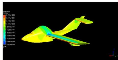
Figure 14 Pressure distribution with  $\alpha = 0^\circ$
