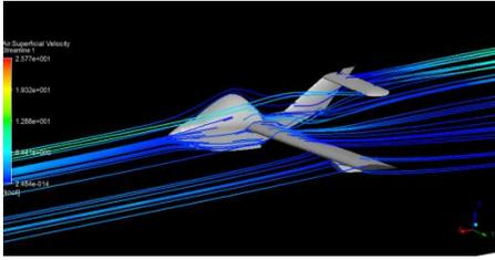
Figure 15 Air velocity streamline with  $\alpha = 0^\circ$
