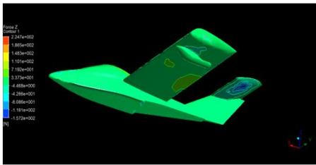
Figure 16 Force Z (lifting) force with  $\alpha = 0^\circ$
