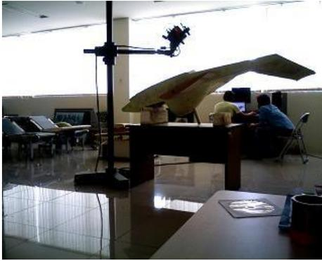
Figure 9 Laser camera photos tracking on the fuselage
