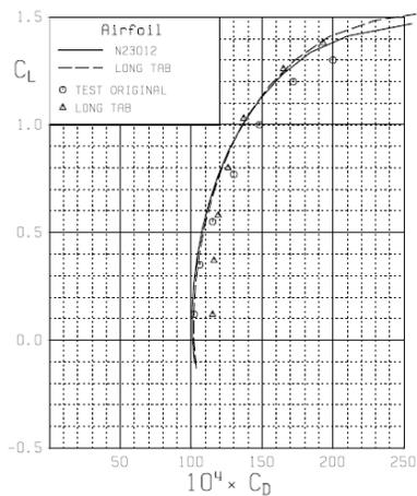
Figure 3 The drag polar of NACA 23012 airfoil<sup>[17]</sup>
