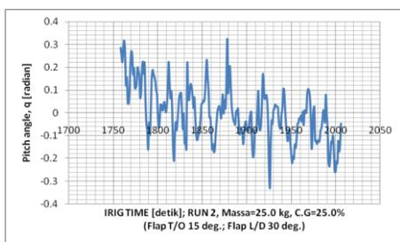
**Figure 21** The Pitch angle,  $\theta$  of Unmanned Aerial Vehicle “Alap alap” flight testing data during takeoff
