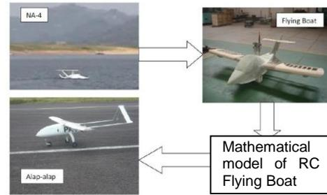
Figure 7 Full configuration of Flying Boat remote control model between NA4 Wing in Surface Effect RC model and Unmanned Aerial Vehicle "Alap alap"
