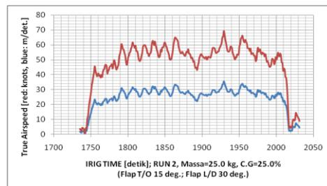
Figure 20 The True Airspeed, V of Unmanned Aerial Vehicle “Alap alap” flight testing data during takeoff
