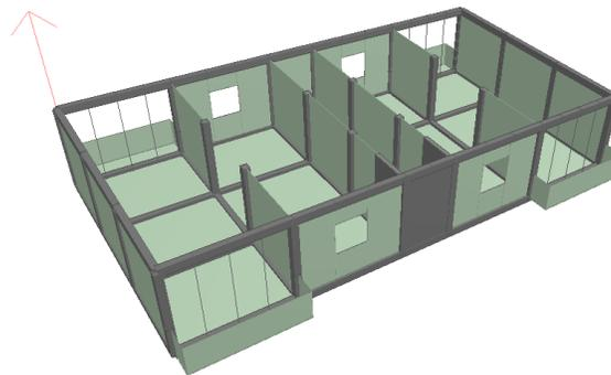
Figure 4 Typical 3-D layout view for each floor
