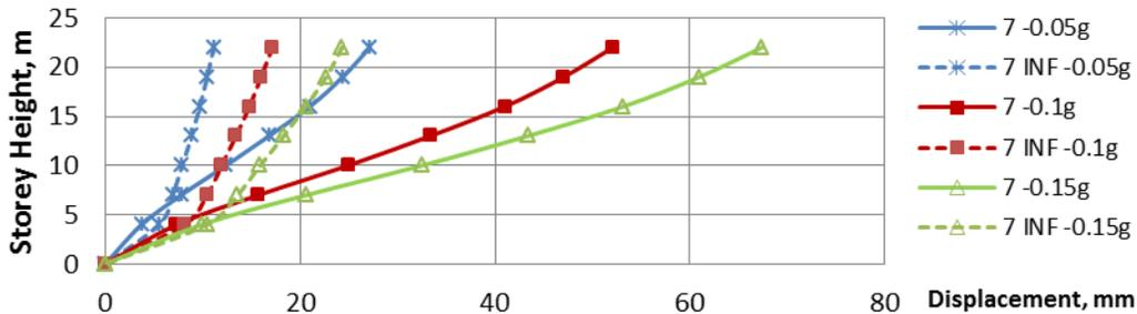
Figure 8 The Maximum lateral Displacements of seven-story Building
