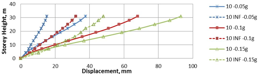
Figure 9 The Maximum Lateral Displacements of 10-story Building
