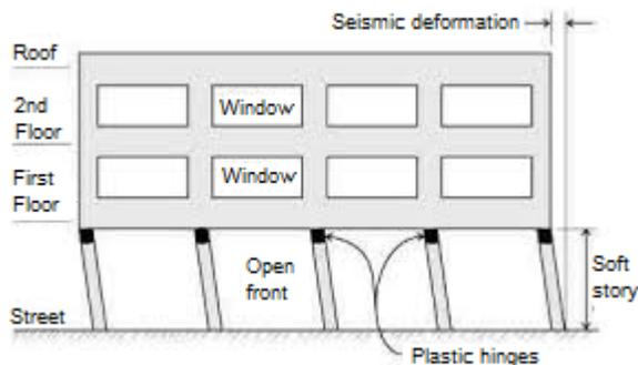
Fig. 1 Soft story mechanism in building
