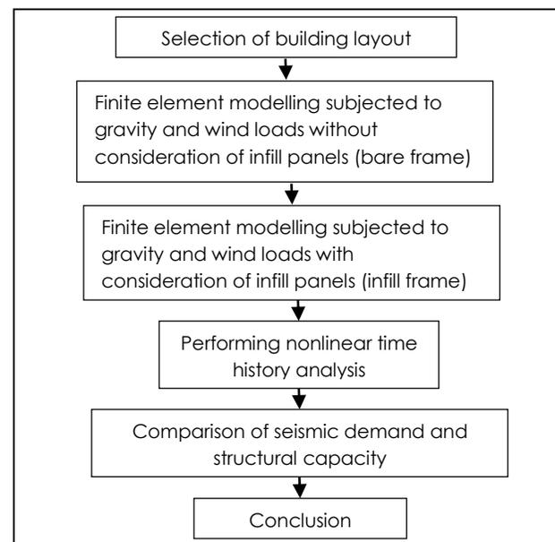
Figure 2 Procedure of analyses
