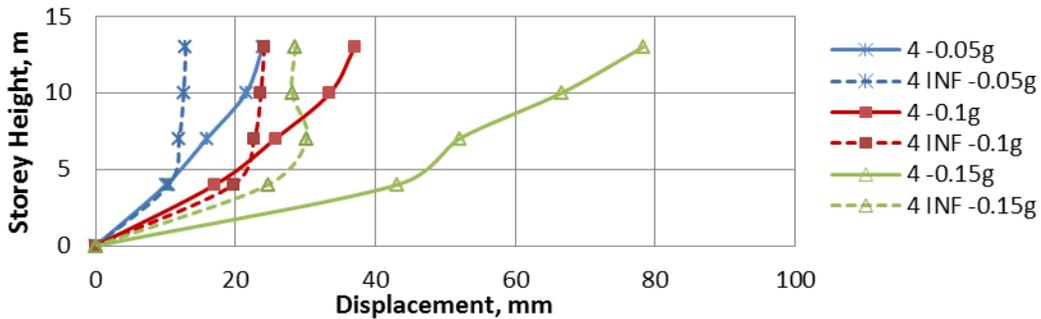
Figure 7 The Maximum Lateral Displacements of four-story Building
