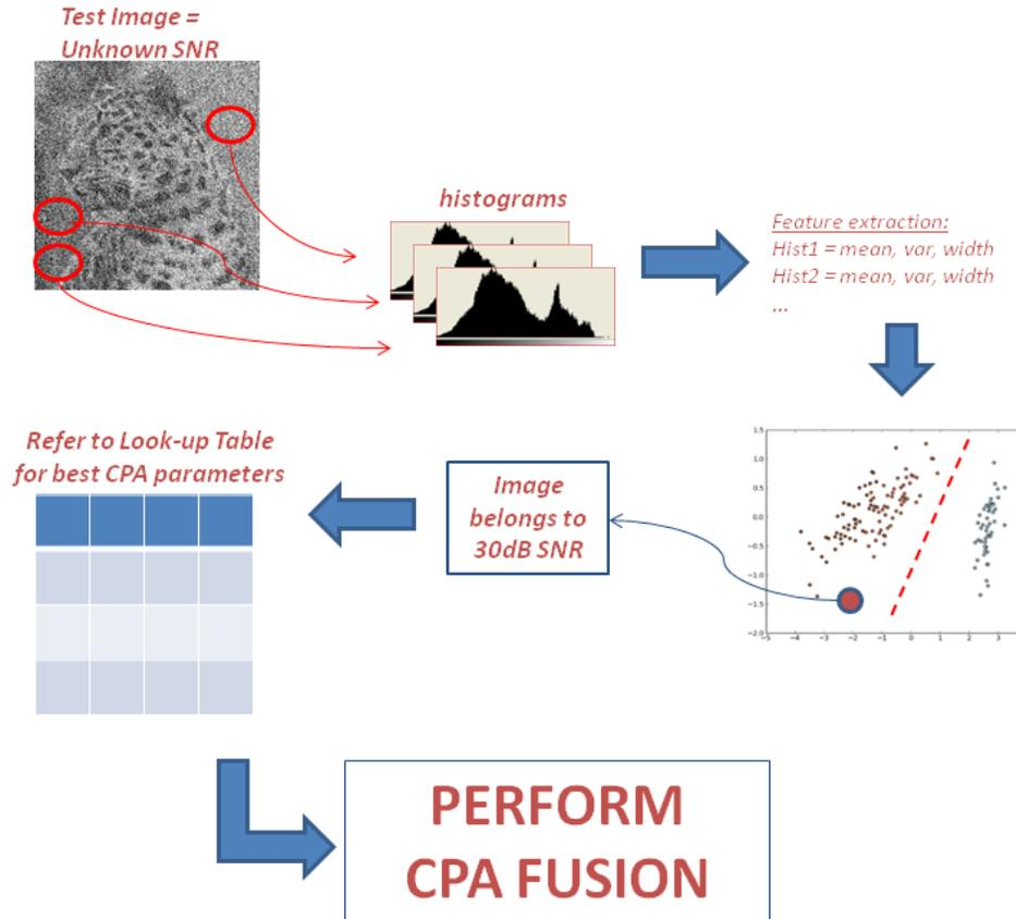
**Figure 2** SVM testing and subsequent adaptive CPA fusion
