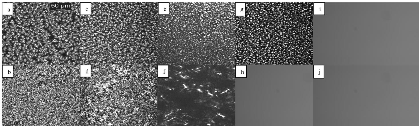
Figure 4 Microstructure images of PS:RBO blends; a) NIE PS100; b) CIE PS100; c) NIE PS70; d) CIE PS70; e) NIE PS50; f) CIE PS50; g) NIE PS30; h) CIE PS30; i) NIE RBO100; j) CIE RBO100 tempered for 20 minutes at 20°C at rate 5°C/min, Magnification 200x and bar represent 50μ
