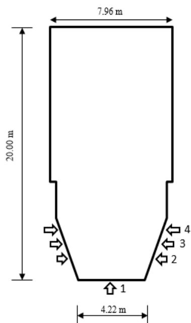
**Figure 1** The fluidized bed reactor system (1) primary air, (2) coal feed, (3) lower secondary air and (4) upper secondary air
