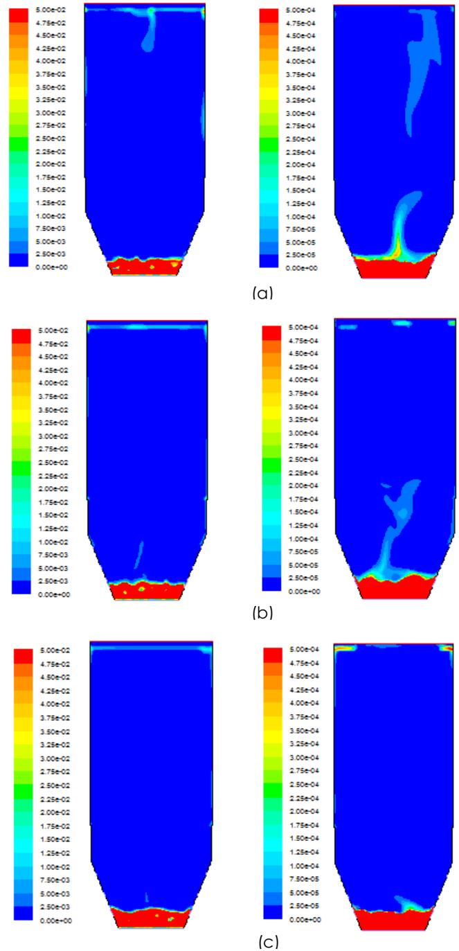
Figure 4 Contours of sand (left) and coal (right) solid volume fractions at 75 s (a) sand 180 μm : coal 500 μm, (b) sand 180 μm : coal 700 μm and (c) sand 180 μm : coal 1000 μm
