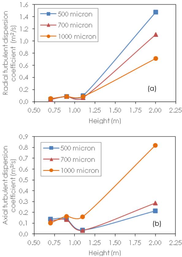
Figure 3 Turbulent dispersion coefficient with different coal solid particle sizes (a) radial direction and (b) axial direction
