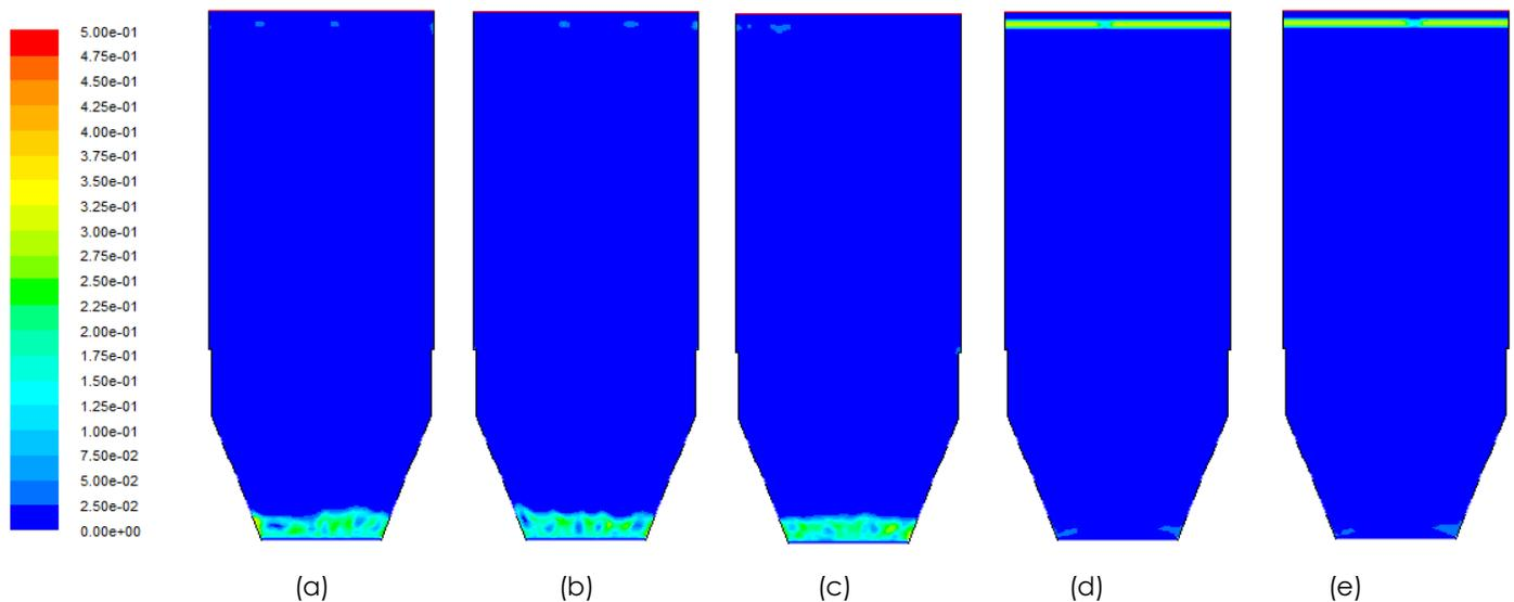
**Figure 2** Contours of sand volume fraction for (a) EMMS drag model at 50 s, (b) EMMS drag model at 55 s, (c) EMMS drag model at 60 s, (d) Gidaspow drag model at 60 s and (e) Wen & Yu drag model at 60 s
