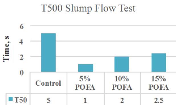
Figure 2 The bar graph of Slump Flow  $T_{500}$  Result
