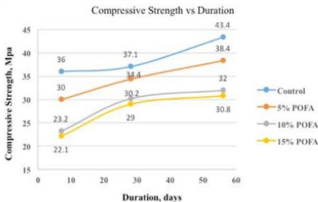
Figure 4 Average value of compressive strength for each type of concrete
