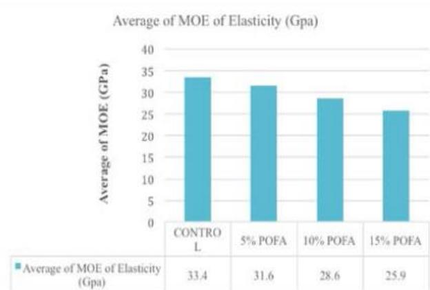
Figure 5 Results of Modulus of Elasticity
