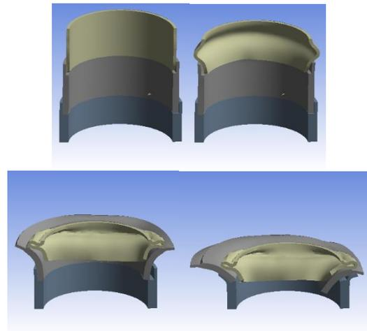
Figure 7 Deformations sequence of three segments crash box (type 1)
