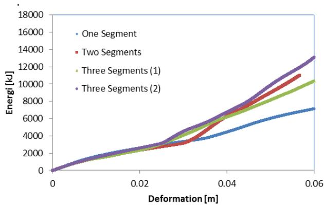
Figure 4 The relation between energy absorbed with deformation for all models of crash box
