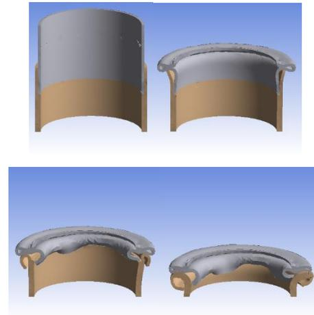
Figure 6 Deformation sequence of two segments crash box
