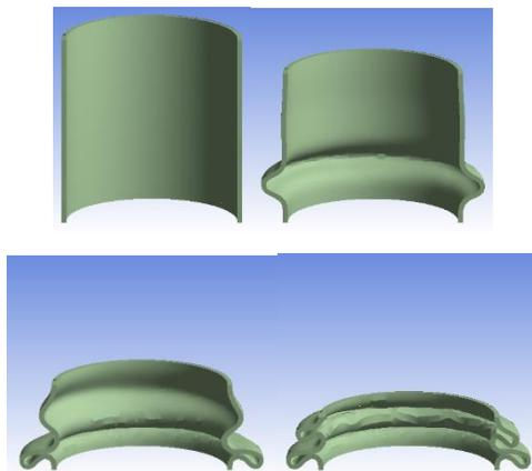
Figure 5 Deformation sequence of one segment crash box
