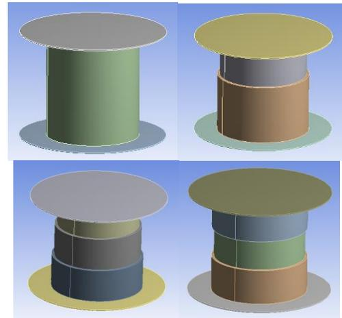
Figure 2 Crash box model: 1 segment, 2 segments, 3 segments (type 1) and 3 segments (type 2)
