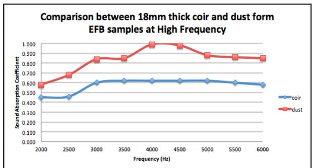
**Figure 8** Sound absorption coefficients of 18mm thick coir and dust form EFB at high frequency region
