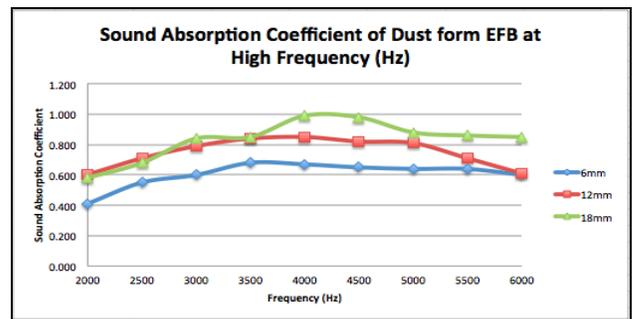
**Figure 5** Sound absorption coefficient of dust form EFB at high frequency region
