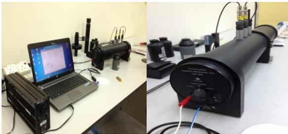
**Figure 2** Impedance tubes
