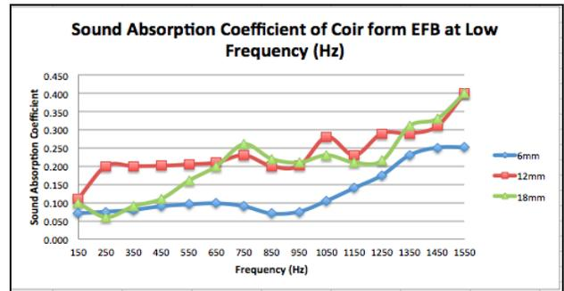
**Figure 4** Sound absorption coefficient of coir form EFB at low frequency region
