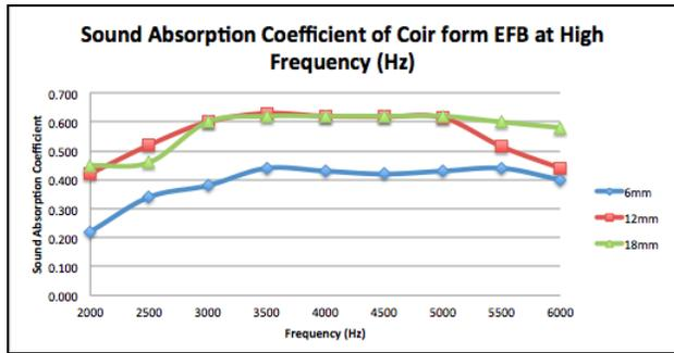
**Figure 6** Sound absorption coefficient of coir form EFB at high frequency region
