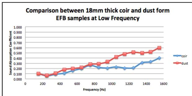
**Figure 7** Sound absorption coefficients of 18mm thick coir and dust form EFB at low frequency region
