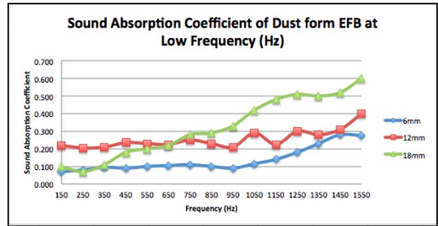
**Figure 3** Sound absorption coefficient of dust form EFB at low frequency region
