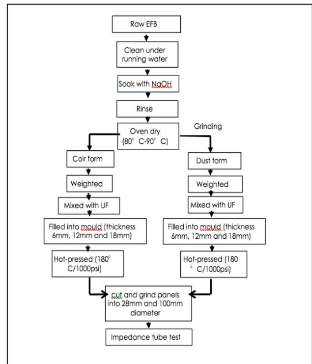
**Figure 1** Process Chart for Sample Preparation
