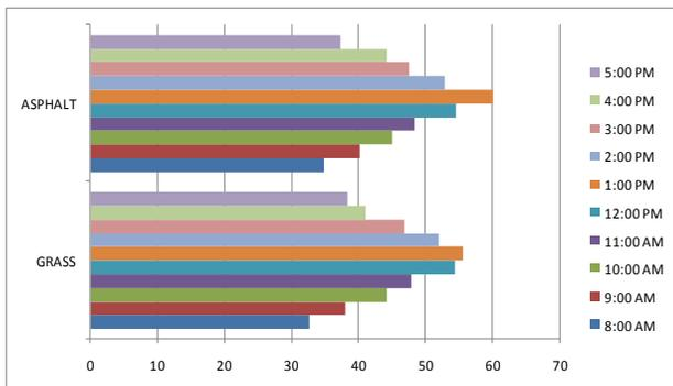
**Figure 11** Surrounding effect on temperature characteristics of grade 5mm paver
