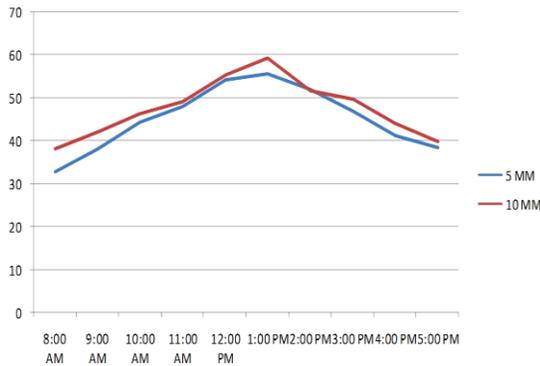
**Figure 9** Temperature and time for paver on grass
