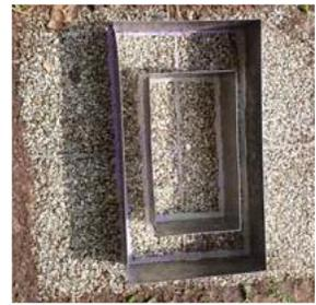
Figure 8 Double ring infiltrrometer
