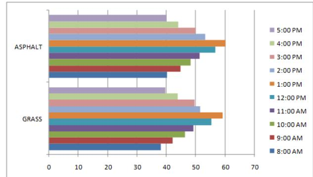
**Figure 12** Surrounding effect on temperature characteristics of grade 10mm paver
