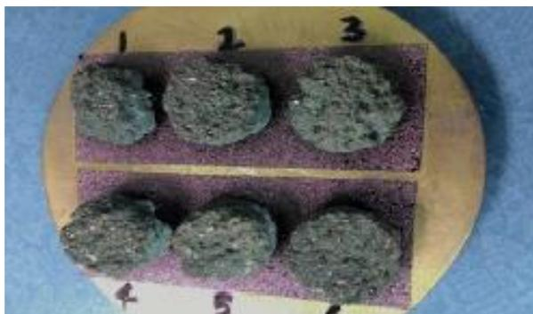
Figure 2 The small pieces of each specimen used to test on SEM
