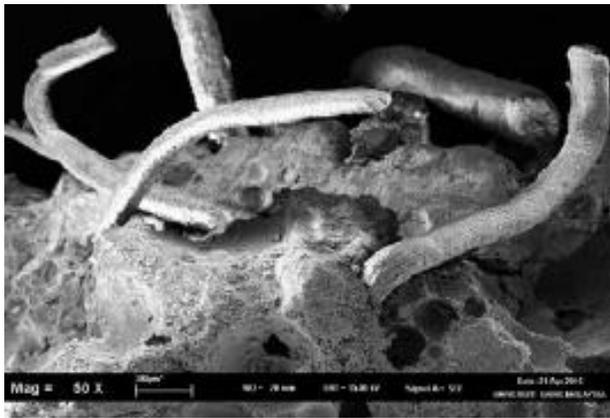
**Figure 7** Scanning electron micrograph showing crack bridging, small holes and long grooves on the fracture surface of LFC (50x magnifications)
