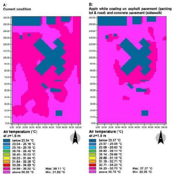
**Figure 9** Air temperature at two different conditions: current condition (A) and modified conditions (B) compared at 15:00 in pedestrian level (1.5 m)
