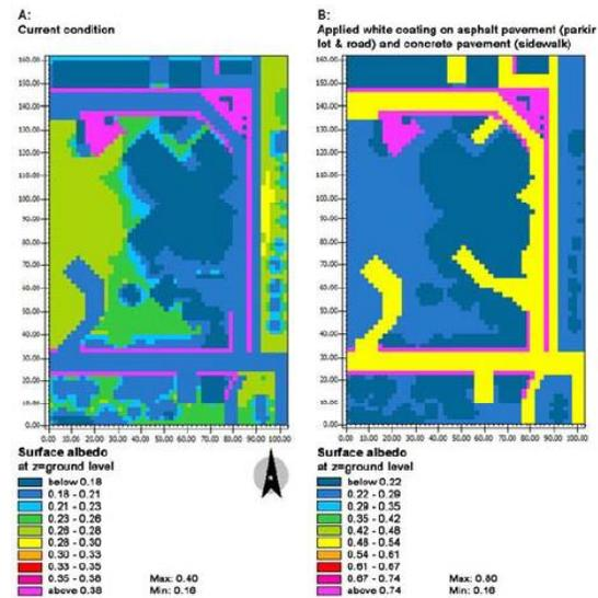
Figure 8 Surface albedo at two different conditions: current condition (A) and modified conditions (B) compared at 15:00 in ground level
