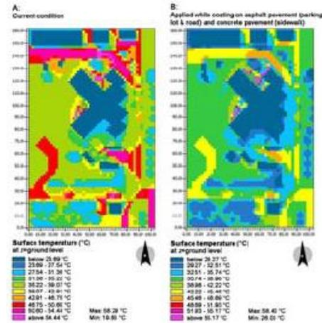
Figure 7 Surface temperature at two different conditions: current condition (A) and modified conditions (B) compared at 15:00 in ground level
