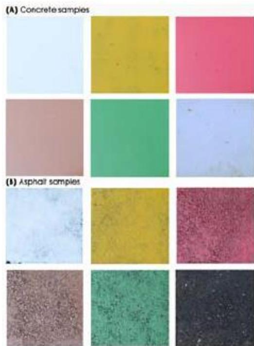
**Figure 1** The color coated and uncoated concrete (above) and asphalt (below) samples
