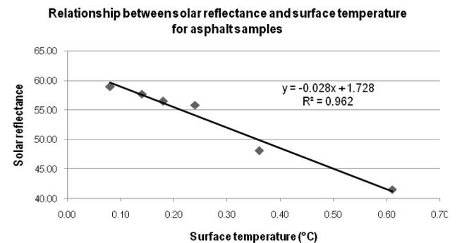
Figure 3 Regression of solar reflectance and surface temperature of asphalt sample
