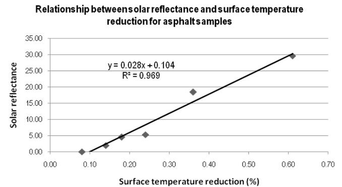
Figure 4 Regression of solar reflectance and surface temperature reduction of asphalt sample
