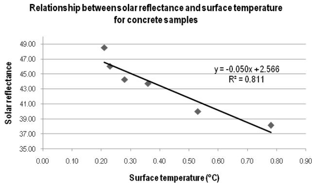
Figure 5 Regression of solar reflectance and surface temperature of concrete sample
