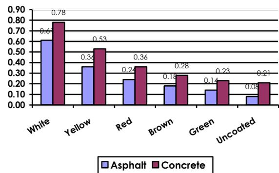
**Figure 2** The solar reflectance of the tested color coated and uncoated for asphalt and concrete samples
