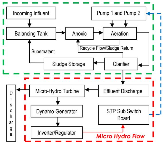
**Figure 5** The ideal application of micro hydro embedded at effluent discharge point of STP.
