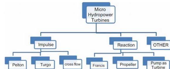
**Figure 3** The classification of Micro Hydro [28]
