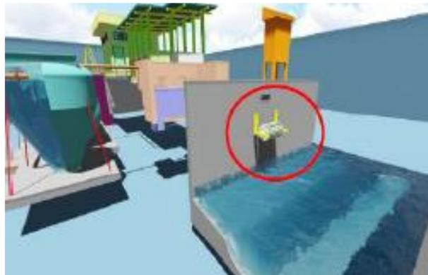
**Figure 2** The effluent discharge pipe to be embedded with a micro hydro at STP (highlighted in circle)
