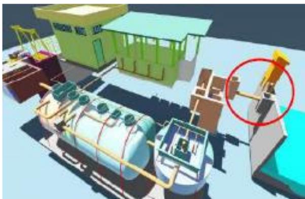
**Figure 1** The location of effluent weir and effluent discharge pipe at STP (highlighted in circle)
