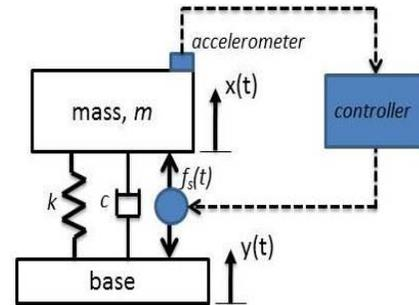
Figure 1 Single-degree-of-freedom model of active vibration isolation system
