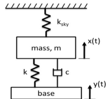
Figure 2 Physical assumption of active stiffness vibration isolation system
