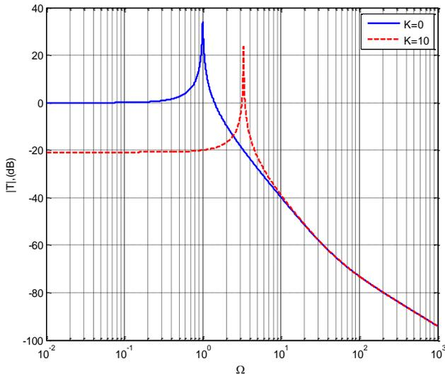
**Figure 3** Comparison of absolute motion transmissibility performance between passive and active stiffness vibration isolation. Blue solid line represents passive vibration isolation system, and red dashed line represents active stiffness vibration isolation system
