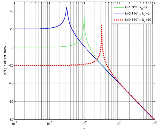
**Figure 5** Comparison of receptance plot for three different configurations. Green line represents fully passive system with stiffness ( $k=1$  N/m), blue bold solid line represents fully passive system with low stiffness ( $k=0.1$  N/m), and red dashed line represents hybrid system with the combination of low passive and active stiffness ( $k=0.1$  N/m,  $k_s=10$  N/m)
