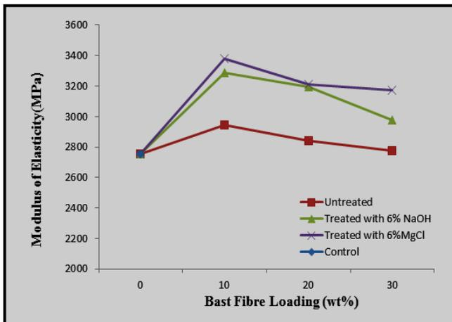
**Figure 4** Average MOE result for untreated and treated kenaf polyethylene composite
