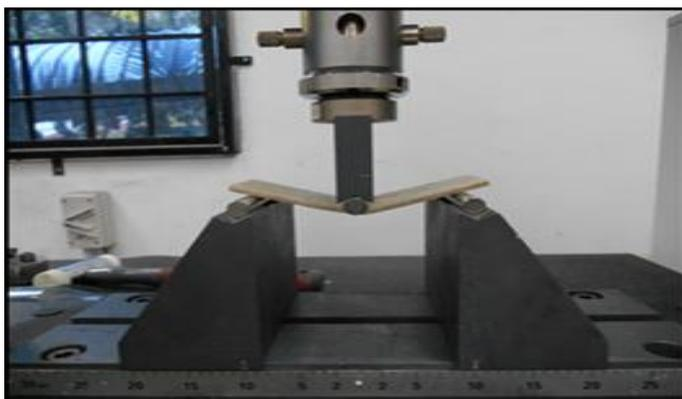
Figure 2 The specimen after bending test
