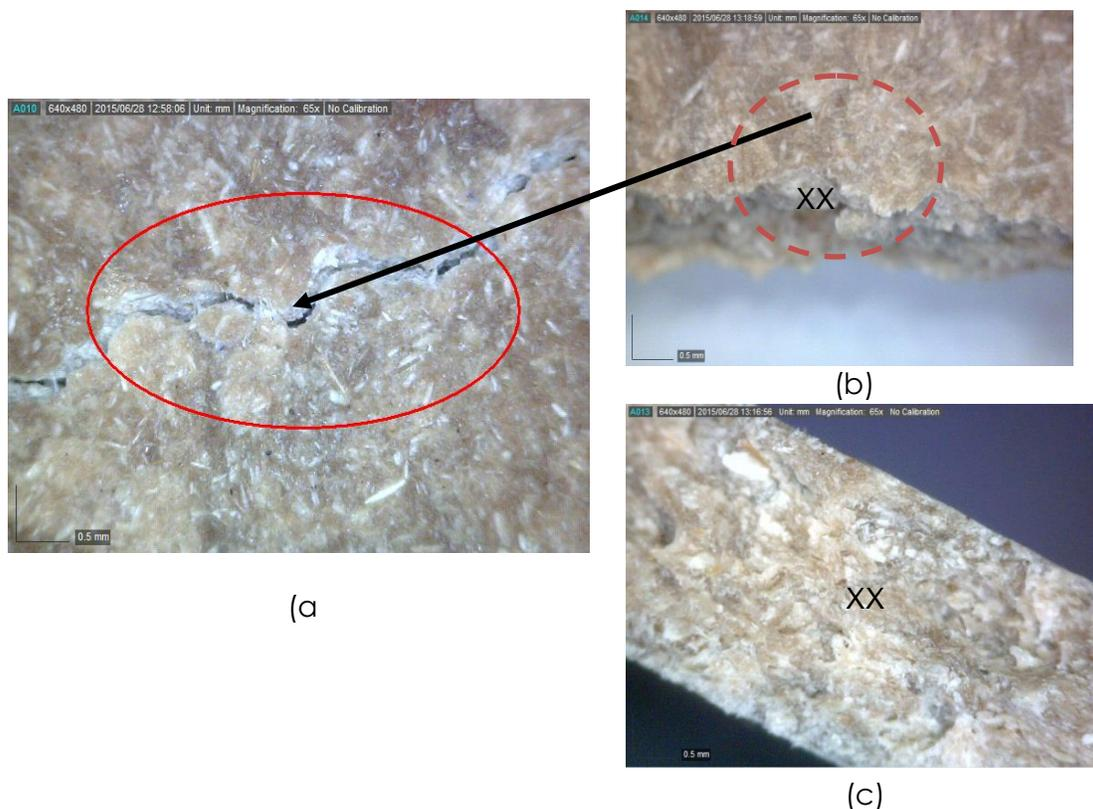
**Figure 5** (a) crack opened (b) location of observation (c) fracture surface failure
