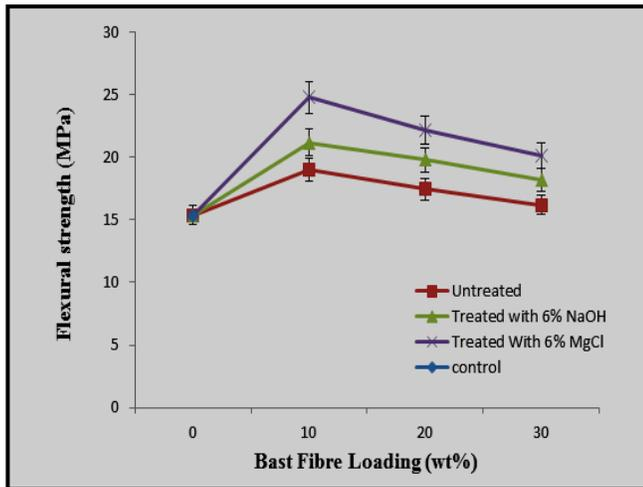
**Figure 3** Average flexural strength result for untreated and treated kenaf polyethylene composite
