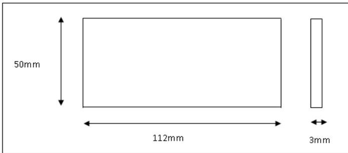
Figure 1 Dimensions of flexural test specimen
