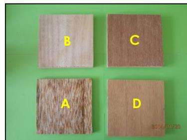
**Figure 1** Different types of plywood; A- PTA, B- PTB, C- PTC, D-PTD
