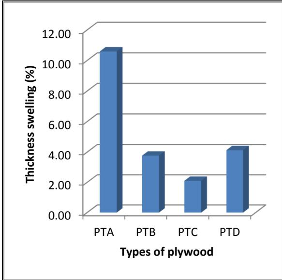
Figure 2 Thickness swellings of all types of plywood
