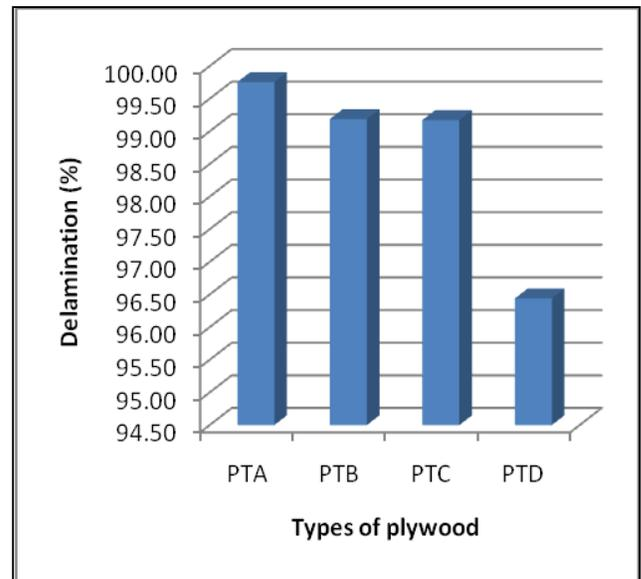
Figure 4 Delamination of all types of plywood
