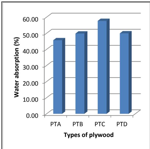
Figure 3 Water absorption of all types of plywood
