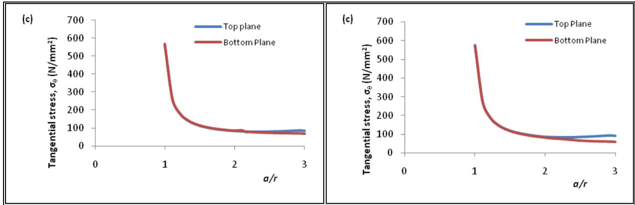
**Figure 2** Comparison of stress distribution at top and bottom plane using PX4 CFRP with  $d= 10$  mm and a nominal stress of 250 N/mm<sup>2</sup> in C-C and C-S configurations. (a) Tangential stress around the hole boundary with clamping force = 500 N (b) Tangential stress around the hole boundary with clamping force = 2000 N (c) Tangential stress on net-tension plane with clamping force = 2000 N
