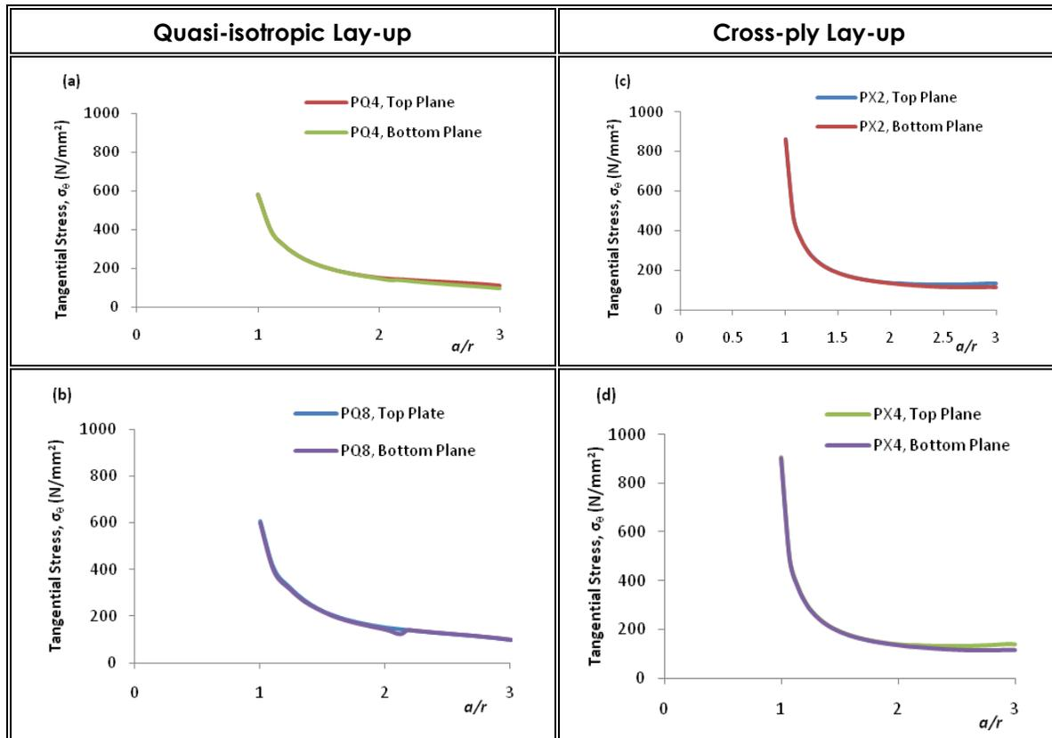
**Figure 4** Comparison of stress distribution in quasi-isotropic and cross-ply lay-ups with  $d=10$  mm on top and bottom plane at an applied bearing stress of  $400 \text{ N/mm}^2$  and clamping force =  $500 \text{ N}$  (a) PQ4, (b) PQ8, (c) PX2, and (d) PX4
