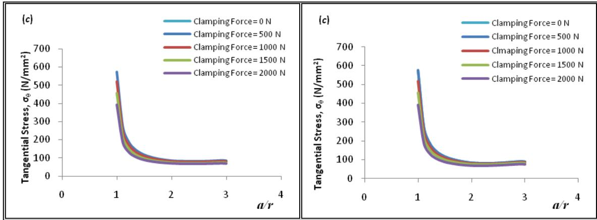
Figure 1 Comparison of stress distributions in C-C and C-S combinations using PX4 CFRP with  $d = 10$  mm and a nominal stress of 250 N/mm<sup>2</sup>. (a) Radial stress around the hole boundary (b) Tangential stress around the hole boundary (c) Tangential stress on net-tension plane
