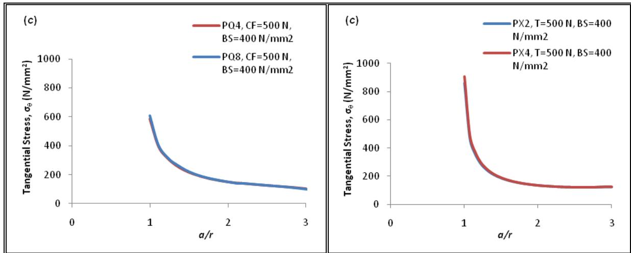
**Figure 3** Comparison of stress distribution in quasi-isotropic (PQ4 and PQ8) and cross-ply (PX2 and PX4) lay-ups with  $d = 10$  mm at an applied bearing stress of  $400 \text{ N/mm}^2$  and clamping force =  $500 \text{ N}$  (a) Radial stress around hole boundary (b) Tangential stress around hole boundary (c) Tangential stress at net-tension plane
