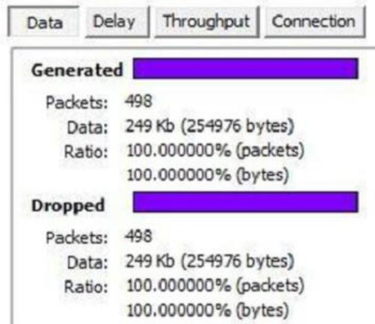
Figure 11 Sink hole attack and Packet drop statistics
