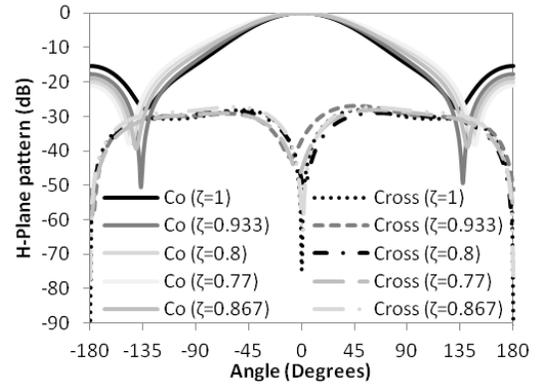
**Figure 5** H-Plane radiation pattern
