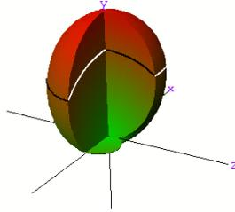
**Figure 3** Three-dimensional radiation pattern of patch antenna
