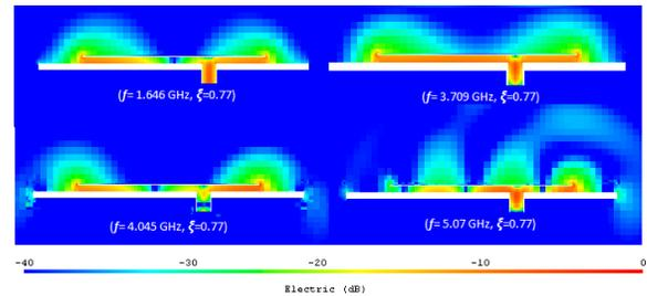
**Figure 7** Space-domain electric field comparison of the crumpled patch antenna ( $\xi=0.77$ ) at different resonance frequencies (viewed in the *YZ*-plane)
