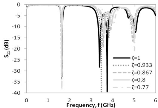
**Figure 2**  $S_{11}$  for different crumpling conditions
