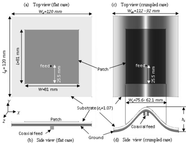
**Figure 1** Flat planar device and an example digitized crumpled antenna
