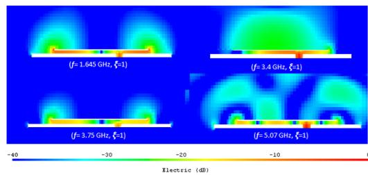
**Figure 6** Space-domain electric field comparison of the un-crumpled patch antenna ( $\xi=1$ ) at different resonance frequencies (viewed in *YZ*-plane)
