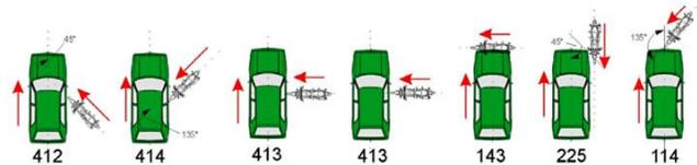
Figure 2 Full-scale crash test configurations as described in ISO 13232 [22]
