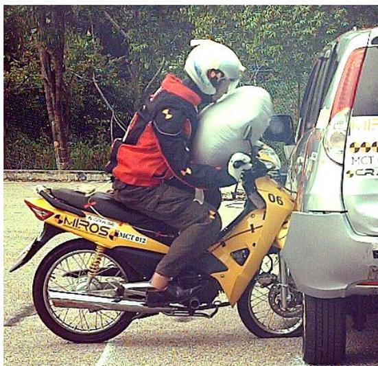
Figure 5 Airbag at full deployment
