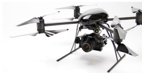
**Figure 3** Unmanned helicopter as traffic sensor[49].
