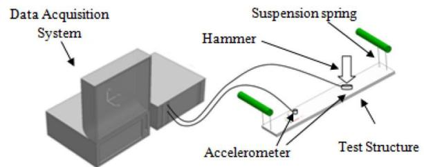
Figure 1 (b) General experimental set-up for free-free boundary conditions
