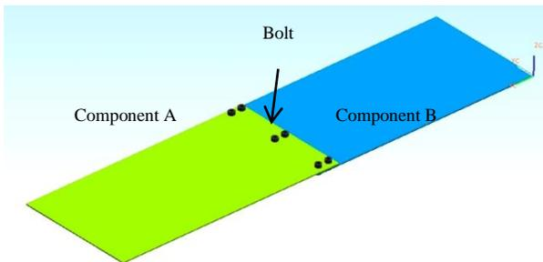
Figure 1 (a) CAD model of the bolted joined structure
