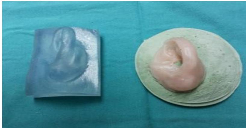
**Figure 8** 3D model of Prosthetic ear from SLA (right) and wax pattern (left) by the maxillofacial technician
