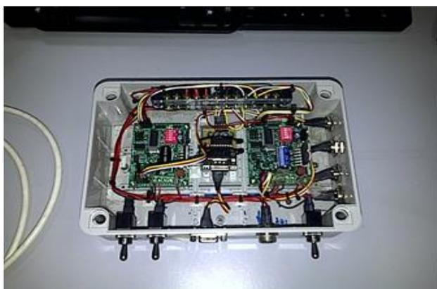
Figure 3 Autotracker control box
