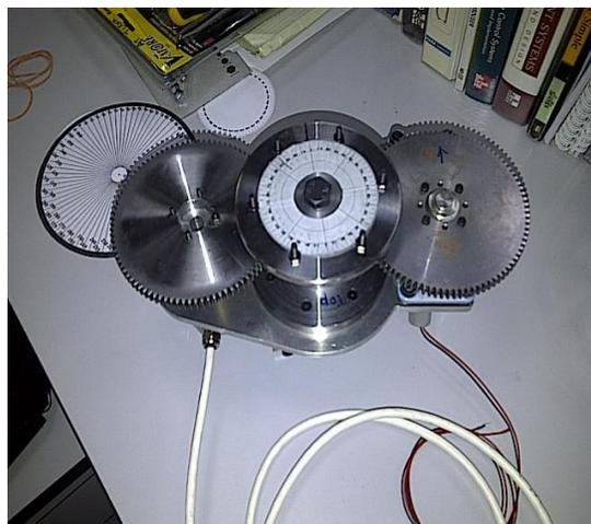
Figure 2 Autotracker Tilt (left) and Pan Mechanism (right)
