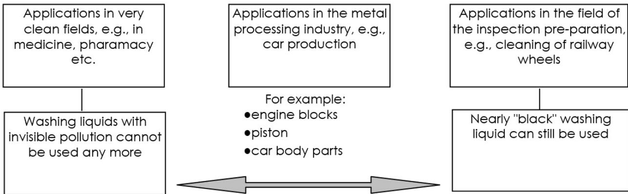
Figure 2 The range of applications of industrial washers
