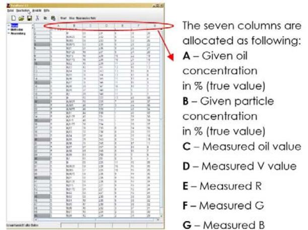
Figure 5 Given out put values and measured input values for teaching the system
