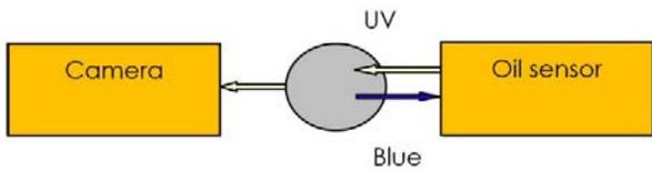
Figure 3 Arrangement of camera and oil sensor at the tube
