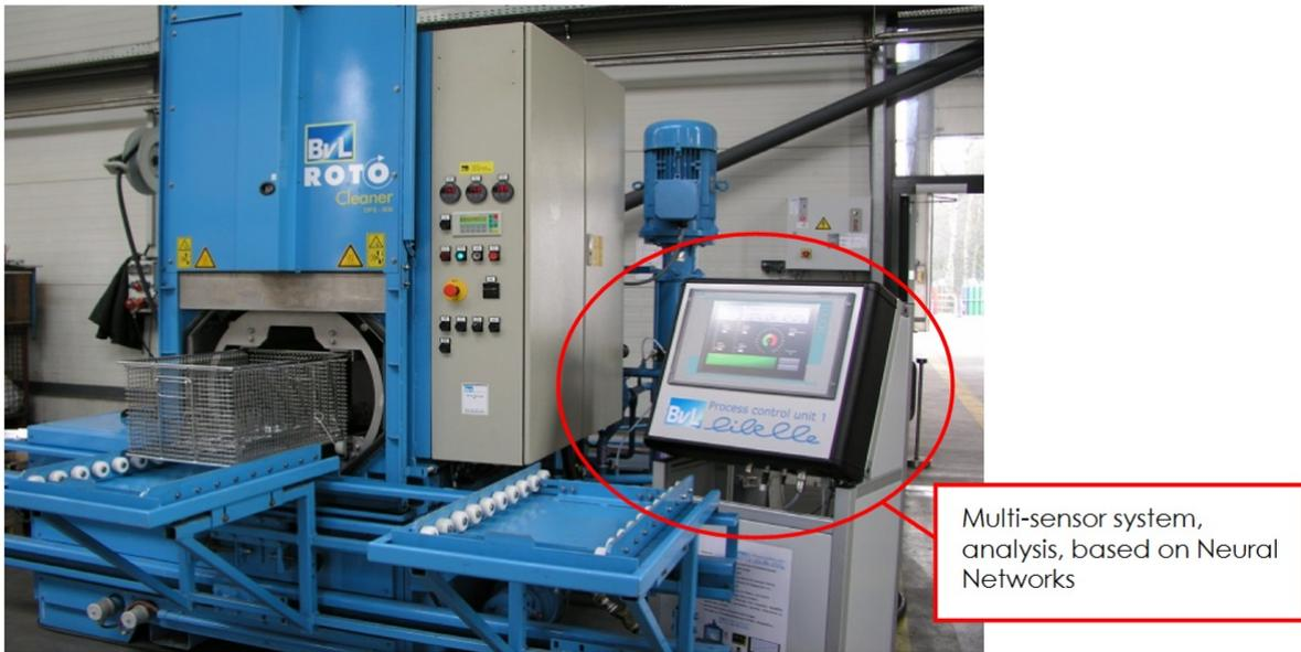
Figure 1 Industrial washer of the company BvLOberflaechentechnik GmbH, Emsbueren, Germany
