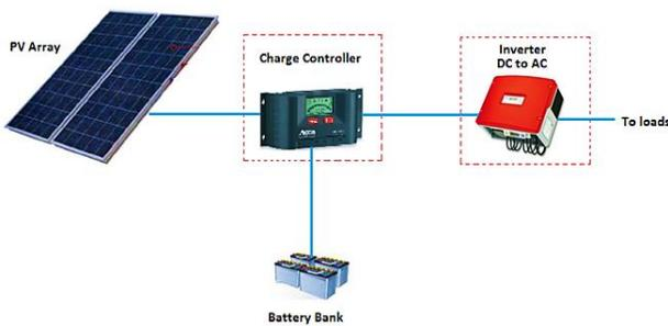
Figure 7 Proposed stand alone solar PV system
