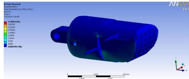
Figure 8 Von-Mises stress - 15N force at z-axis
