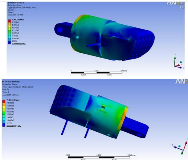
Figure 10 Von-Mises stress - 10N force at y-axis
