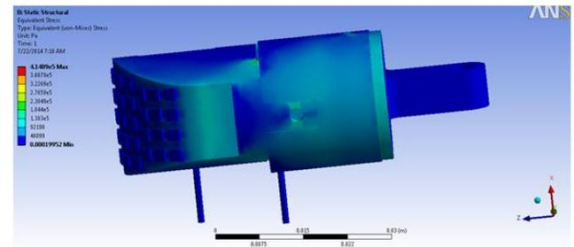
Figure 7 Von-Mises stress - 10N force at z-axis
