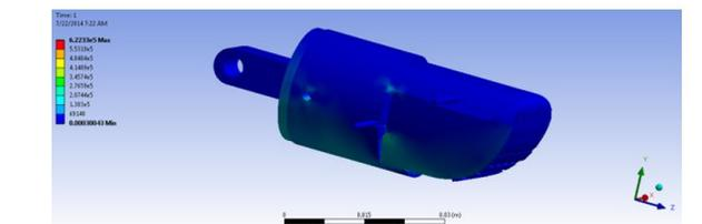
Figure 9 Deformation - 10N force at y-axis
