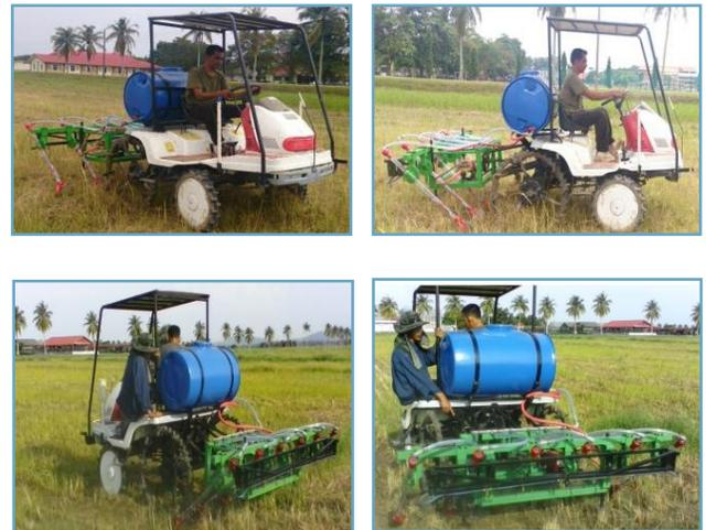
**Figure 3** Field test of the AeRoller machine on weeds at Aerobic rice plot in MARDI Seberang Perai
