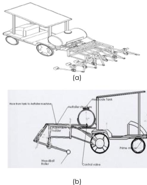
**Figure 2** a)Design of the AeRoller, b)Component and function of the AeRoller
