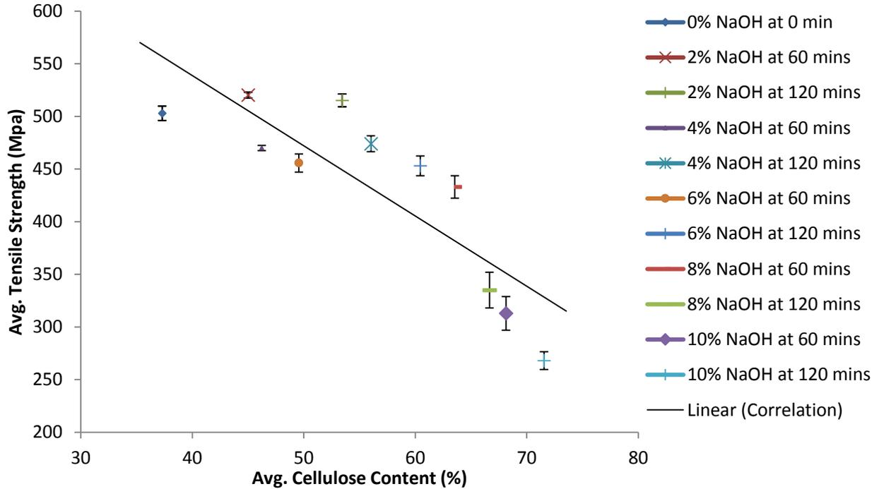
Figure 1 The relationship between cellulose content and tensile strength of continuous single fiber
