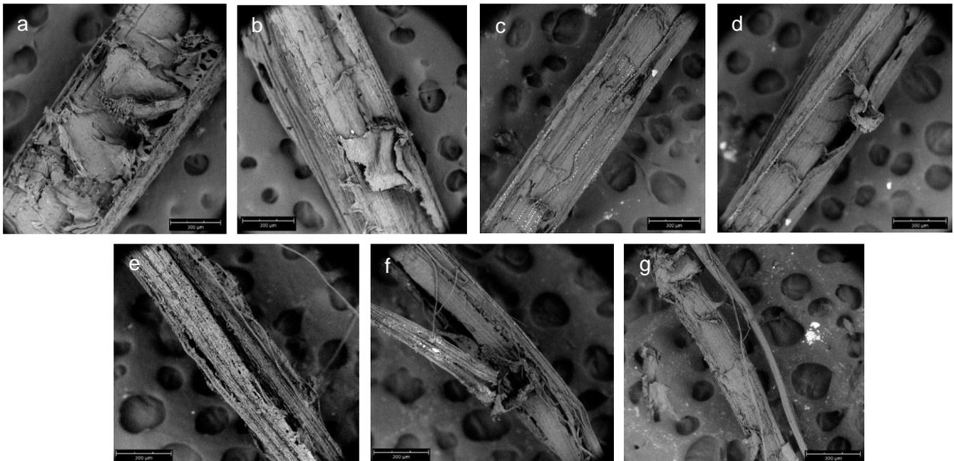
Figure 2 Morphology of single mengkuang fiber before and after each extraction process: (a) 0% Treatment (b) 2% NaOH at 60 min (c) 2% NaOH at 120 min (d) 6% NaOH at 60 min (e) 6% NaOH at 120 min (f) 10% NaOH at 60 min (g) 10% NaOH at 120 min (all magnification at 50x)
