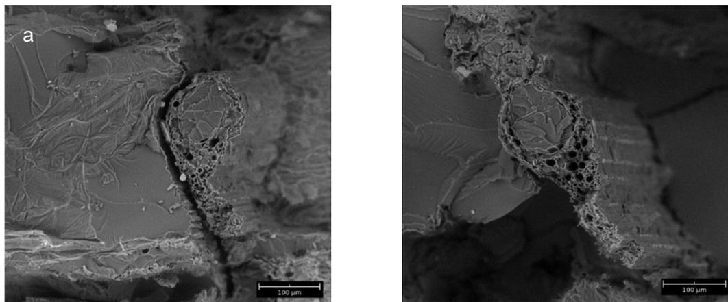
**Figure 3** Morphology of the fracture surface of the continuous Mengkuang fiber composite. (Magnification of 500x)
