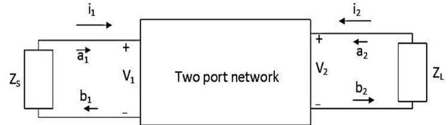
Figure 2 S-parameters representation of a two-port network.
