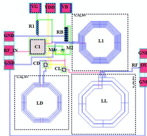
Figure 12 Layout of the proposed LNA (0.93 mm x 1.02 mm)
