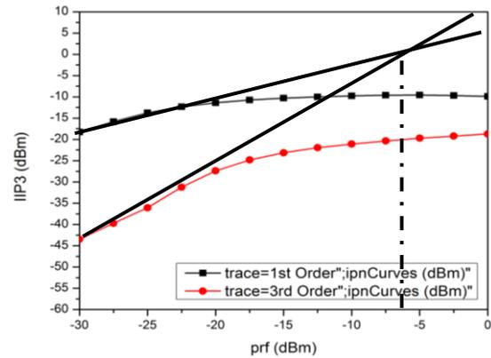
Figure 10 Simulated result of the IIP3
