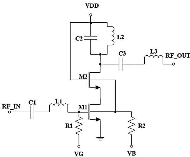
Figure 4 Schematic of the proposed LNA
