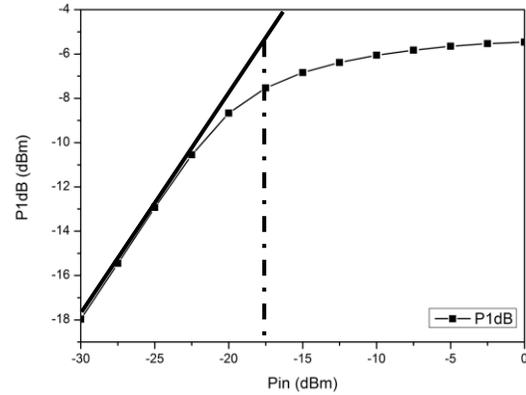
Figure 9 Simulated result of the input 1 dB compression point
