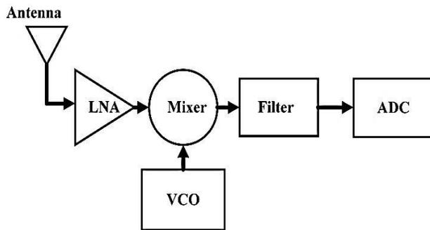
Figure 1 WSN receiver block diagram
