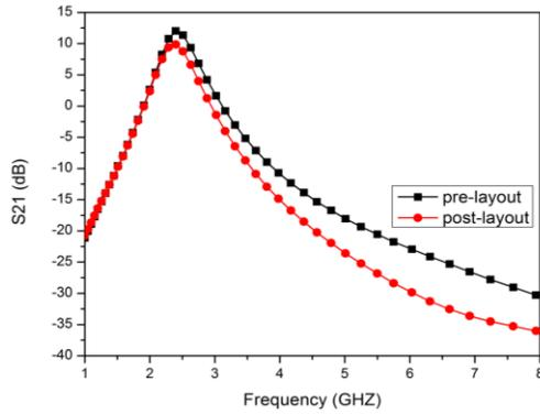
Figure 7 The gain of the proposed LNA
