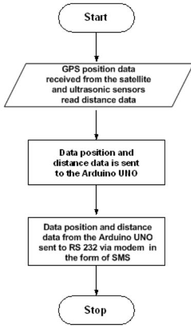
**Figure 7** Position and height data sending through Wavecom Fastrack modem flowchart
