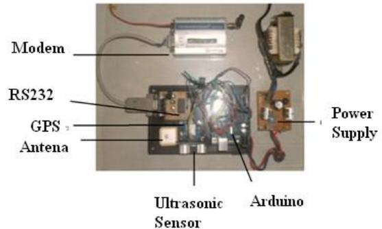
**Figure 9** Device 1 Arduino UNO connected to Wavecom Modem used to send data through SMS
