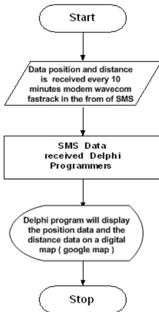
**Figure 8** Position and height data retrieving through Wavecom Fastrack modem flowchart
