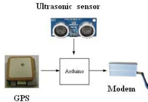
Figure 6 GPS transmitting system and ultrasonic sensor through Wavecom Fastrack modem.
