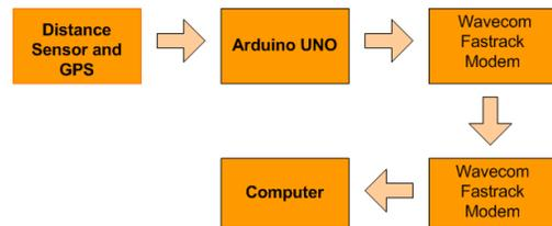
Figure 13 Block diagram of the processes of the system
