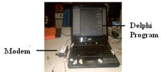
**Figure 10** Device 2 Wavecom modem connected to a PC Used to receive data sent from device 1
