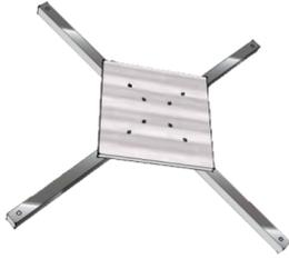
Figure 3: Cross structure of the developed quadcopter frame
