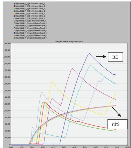
Figure 6: Average throughput of rtPS and BE for 15 mobile nodes
