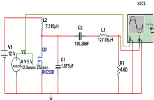
Figure 3: Class-E converter design circuit
