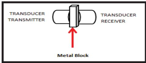
Figure 11: Positioning Of Metal Block between Transducer Transmitter And Receiver
