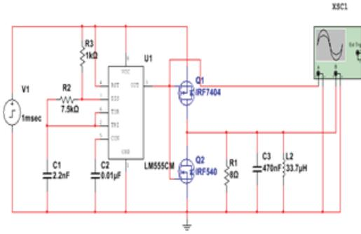
Figure 2: Push-Pull converter design circuit
