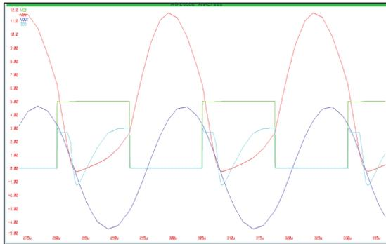
Figure 8: ZVS condition for Class-E circuit
