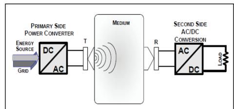
Figure 1: The basic principle of APT system
