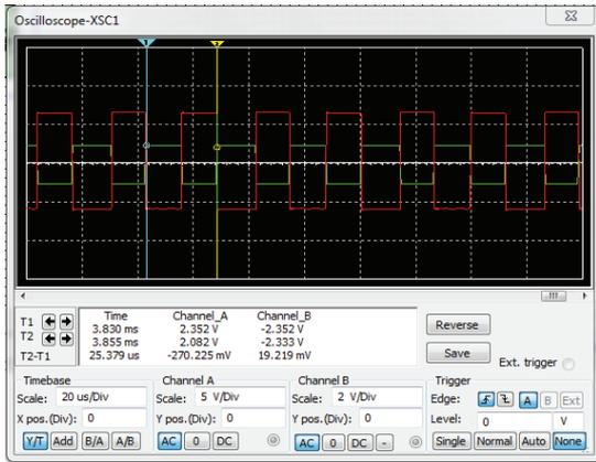
Figure 5: Oscilloscope output at f = 40 kHz (Ch. A – VGS, Ch. B – Output)
