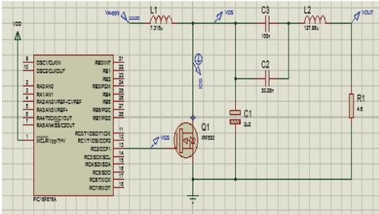
Figure 7: Constructed Circuit Class-E and PIC 16F877A in Simulation
