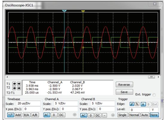
Figure 6: Oscilloscope output at f = 40 kHz (Ch. A – VGS, Ch. B – Output)
