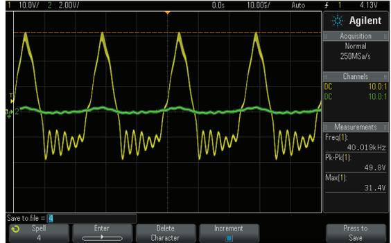
Figure 12: Oscilloscope Result Taken After Metal Block At The Transducer Receiver
