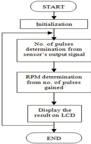
Figure 5: Programming Algorithm of Microcontroller
