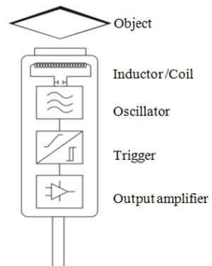
Figure 1: Block Diagram of Conventional Inductive Proximity Sensor
