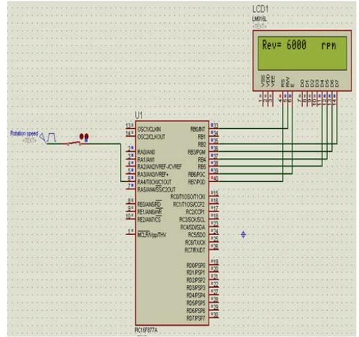
Figure 6: Schematic Circuit Diagram of RPM Measuring System
