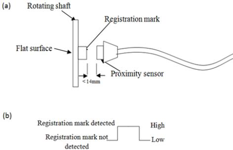
Figure 2: (a) The Placement of Proximity Sensor for Rotational Speed Measurement (b) Pulse Generated (Ideal)
