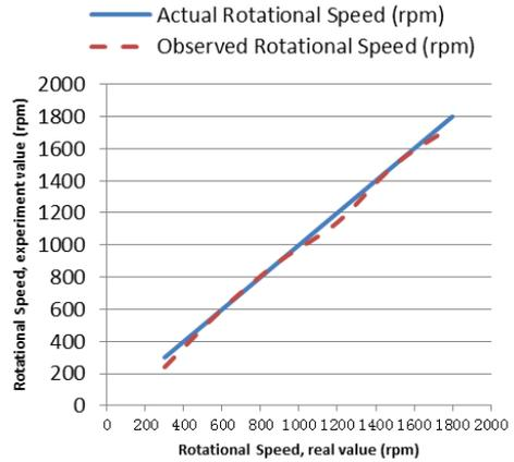
Figure 9: Experimentally Observed Rotational Speed by Proximity Sensor
