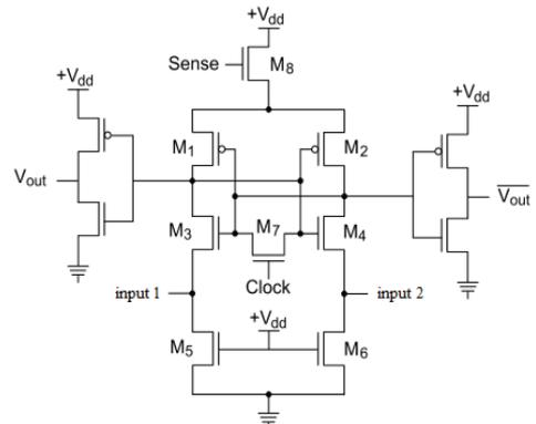
Figure 5: Hybrid current-voltage sense amplifier
