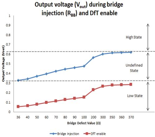
Figure 7: Graph comparison of output voltage ( $V_{out}$ ) during bridge injection ( $R_{BB}$ ) and DfT enable
