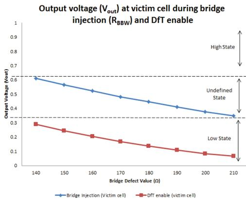
Figure 9: Graph comparison of output voltage ( $V_{out}$ ) at victim cell during bridge injection ( $R_{BBW}$ ) and DfT enable
