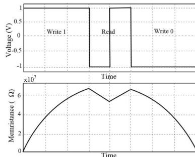
Figure 3: Changes in memristance due to voltage versus time [6]
