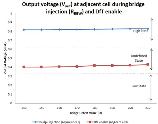
Figure 10: Graph comparison of output voltage ( $V_{out}$ ) at adjacent cell during bridge injection ( $R_{BBW}$ ) and DfT enable
