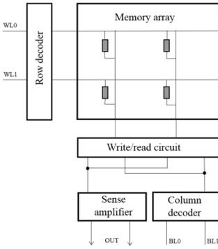
Figure 1: Functional model of ReRAM [7]
