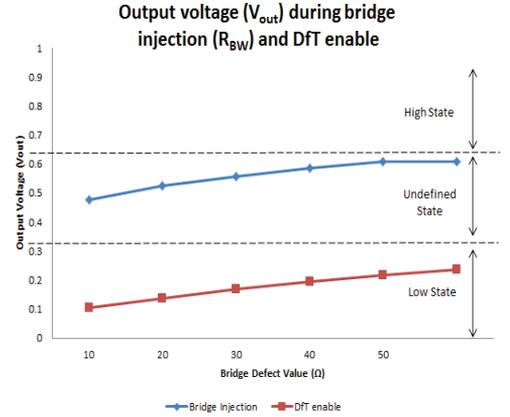
Figure 8 Graph comparison of output voltage ( $V_{out}$ ) during bridge injection ( $R_{BW}$ ) and DfT enable
