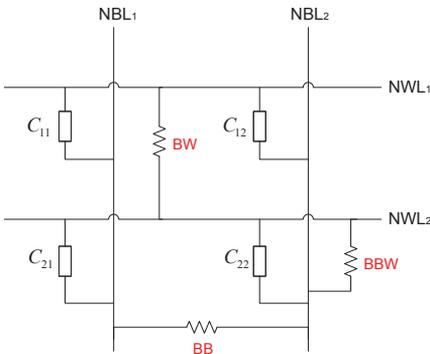
Figure 4: Possible locations of bridge defect
