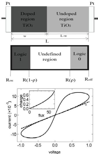
Figure 2: Memristor: (a) model (b) I-V curve
